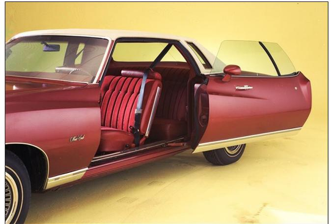
"Personal Luxury Cars" such as the big Monte Carlo had large, heavy doors, and getting in and out of such coupes could be a challenge in tight quarters or where the car is parked on an incline. This sliding-door concept made access into both front and rear seats much better, but it never entered production due to the cost and complexity of the slide mechanism.
