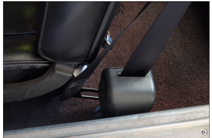
Morris Classic retractor mounted at the factory outer seat belt mount.
