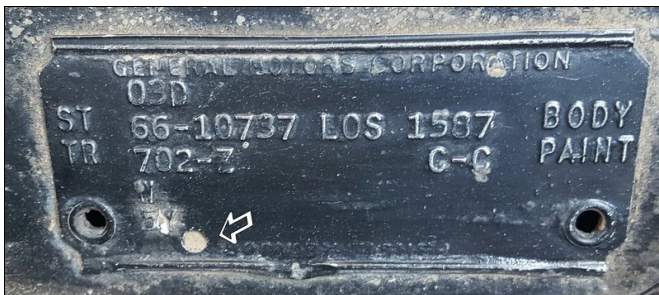
A 1966 body tag with the punched hole (indicated by the arrow) which denotes the presence of the factory shoulder belt mounting points.
