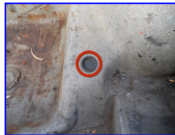
Circled in red, the access plug for the steering box adjuster in the Corvair trunk.
