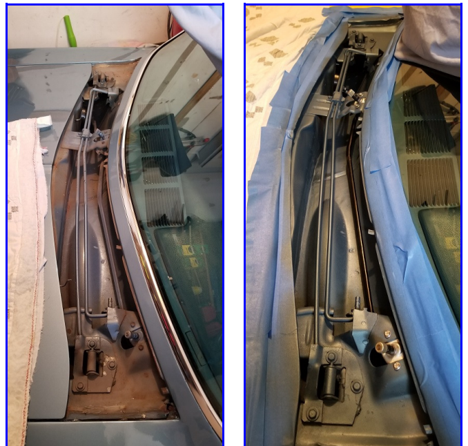
Above, the new linkages and the new motor. Below, before (left) and after (right).
