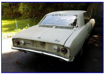
110-hp engine, Powerglide automatic transmission. It's a rusty car, but the structure is solid, with a solid trunk, solid door pillars, solid suspension mounting points. There is rust around the windshield and backlight (as per usual) and there is rust on bottom front fenders, but neither is a difficult fix. Greg says "The floors need some patching though I have owned far worse!" The interior is original and in desperate need of cleaning.
