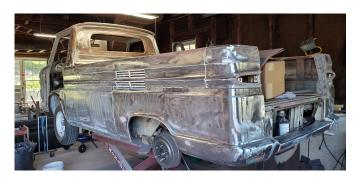
Every bit of white paint has been removed by sanding or sandblasting or by chemical stripping. It's down to bare metal and I'm almost done with the dent repairs which will allow me to soon begin spraying the 2-part epoxy primer... everywhere the paint used to be. The bed floor and the step up for the transmission cover and the engine cover will be addressed soon.
