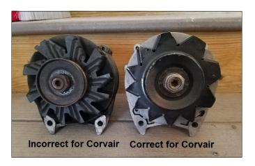
An alternator fan, whether it is designed for clockwise or counter-clockwise rotation, is a centrifugal blower, drawing air from its center and blowing it out radially. Air is drawn in the back of the alternator, pulled through the alternator, and blown out the front by the fan. When run in the reverse direction from its design, as was the case with the incorrect fan on my car, the fan is very, very inefficient. The alternator will overheat.
