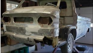
The areas inside of the bed that had white paint and the back of the cab have been stripped.
