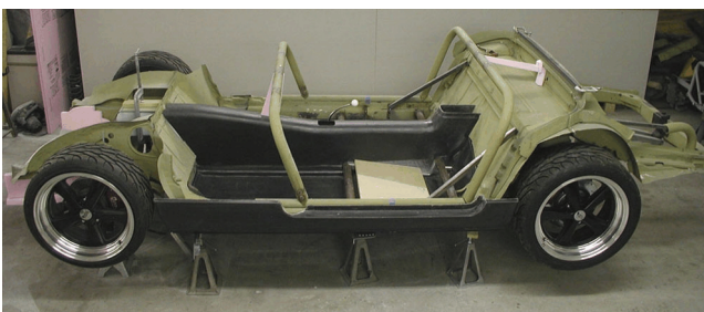
The tolling platform prior to body fabrication
