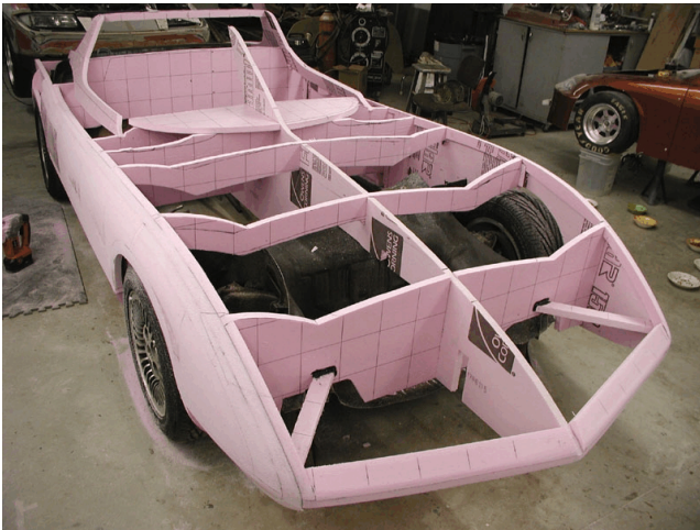
The body shape is mocked up with foam panels
