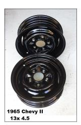
For Sale: Refurbished original wheels from a 1960s Chevy II, 13-inch, same 5-bolt pattern as the 1965-69 Corvair but much narrower, just 4 inches wide as compared to the Corvair's 5.5 inches. Sandblasted and painted, round and true. I bought them to use on the front of my 1966 Corvair for the NECC drag races, but as it turned out I did not
