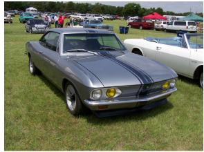
My lastest modification was a carbon fiber deck lid from Bruce Carlton. This shaved about 50 pounds from the rear of the car. I also removed the heater and relocated the battery to the trunk. I also had the car painted, silver with a dark blue Stinger stripe.
