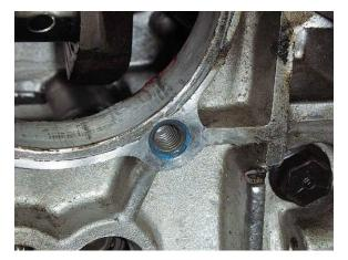
To install the stud to its proper length I use Clarks installation tool (C11310) which uses a steel ball inside a large nut to keep it from tightening up and a set of sleeves to set the height for long or short studs. It works well. I use thread locker on the stud when I reinstall it. I do use anti seize on the head nut threads plus the acorn nuts to protect the exposed threads so the next time it will come apart like it should.
