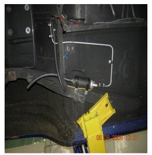
required at full power. The excess fuel has to go somewhere so a return line needs to be installed. It can be made from another Corvair fuel line or fabricated from aluminum line or flexible AN line. There are returnless systems which use bypass pumps but I chose to use the return type to avoid potential hot soak problems. The picture shows the fuel pump mounted position. Please don't use steel line as pictured as it will transmit all of the fuel pump
