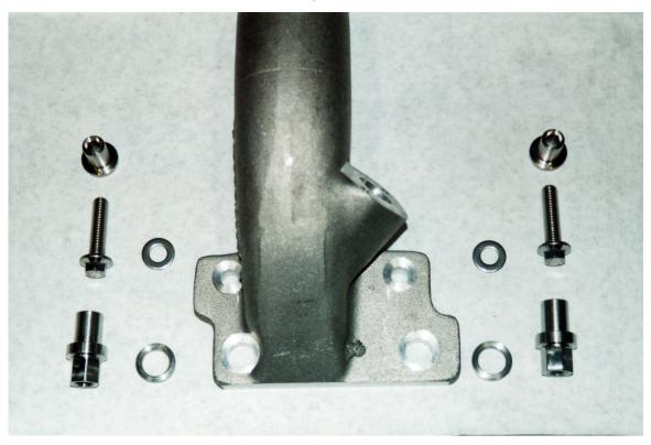
This is the intake manifold (one of 6) and its associated attaching hardware to include upper threaded insert, bolt and washer. The head nuts have a long shoulder which indexes the manifold to its respective port. All of these fasteners are made of stainless steel.
