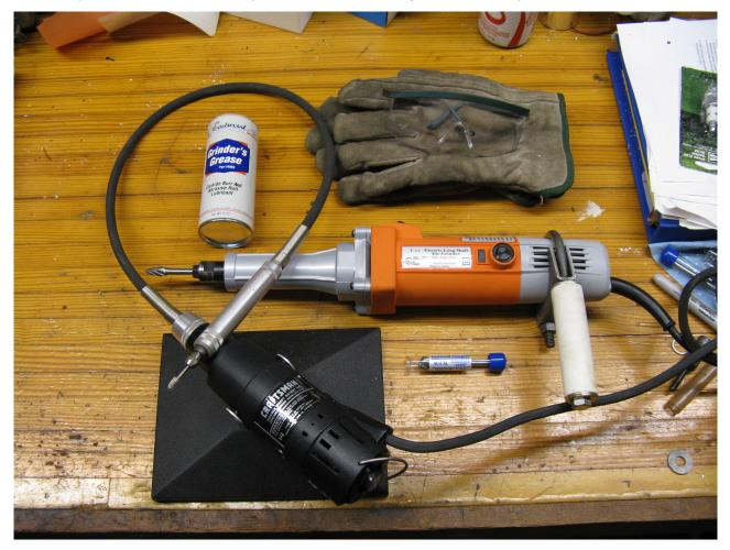
Clockwise from top left: Safety glasses and gloves (the grinder gets hot), Long reach electric die grinder from Harbor Freight, Carbide barrel shaped aluminum burr from Eastwood, Craftsman (Dremel) flex shaft moto-tool, Grinder's Grease also from Eastwood (essential to keep bits from clogging).
