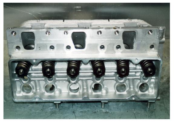
Note the countersunk areas at each head stud this allows for the head nut, with its extended shoulder, to center the manifold on the port. Note also the upper threaded inserts that attach the manifold at its upper edge. Each port is matched with its respective manifold so they become a non divisible pair.
