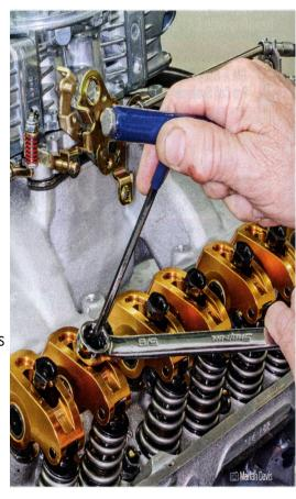
Running tight plunger-to-retainer clearances can be risky if using standard lifters that have a paperclip-type retaining ring because hydraulic pressure may cause the plunger body to pop out of the groove, resulting in catastrophic failure.
