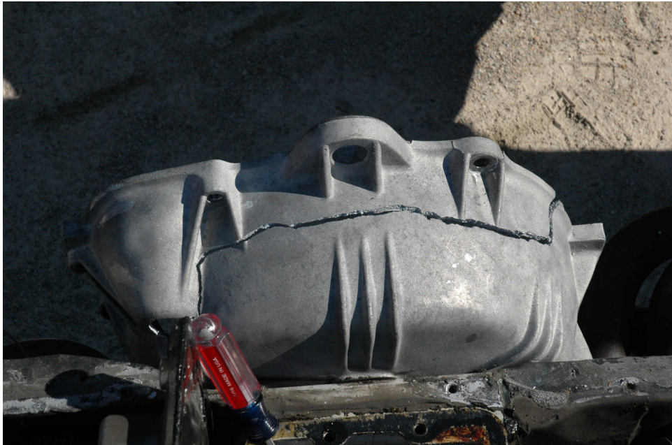
The fly wheel and clutch wobbled hard enough to break the bell housing.
