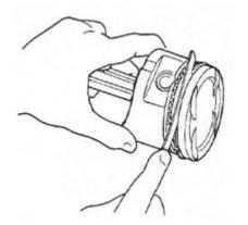
Install a new piston ring backwards into the top ring groove. Insert the largest thickness feeler gauge that fits between the ring and groove. If the thickness exceeds .006" (0.15mm), replace the piston.
