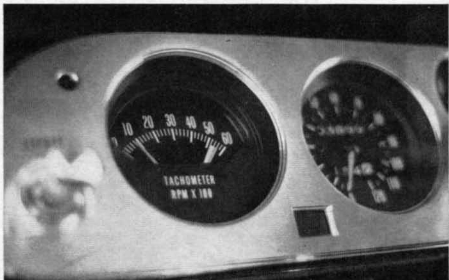
Brushed-aluminum dash is handsome, with nearly complete set of instruments, but markings on tach are too small for quick readings; full-circle dial would help.
