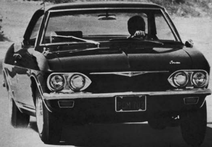
Sonny Balcaen gets his Corvair Corsa a bit out of shape while testing his hop-up and handling kit. A switch to 14-inch Cragar alloy wheels improved the handling as well as giving a slight ratio increase. The 15 to 16 extra horses give plenty of go.
