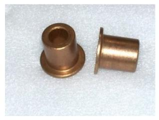
10. Because our cars are now around 50 yrs old, chances are your shift rod is bowed and the bushing will not slide on it easily. To remedy this, simply sand out the inside of the bushing a little. I used a Dremel with a sanding band on it. It doesn't take much, just run it around the inside for a minute or so. It will then slide on your shift rod easily. Don't take too much off, or it will defeat the whole purpose of getting nice, tight shifting.
