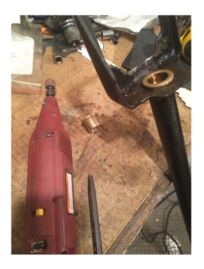
11. You can now install one bushing on each side of the shift tube. In order to really make sure the new brass bushings stay put, you can take a punch and give a tap on the shifter tube to 'stake' the brass bushing in place. (You can see in my photo where I placed a cent er punch on the tube and gave it a good tap)
