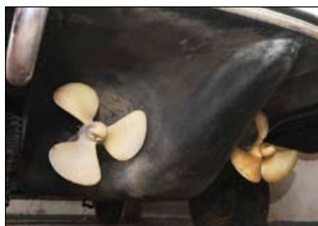
It looks like something Q might fashion for James Bond — the undercarriage of the Amphicar features two propeller for water use.
