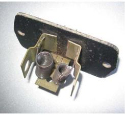
high-resistance resistor, so both resistors are in series with the blower motor. The resistors are mounted away from the board on light heat sinks.
