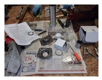
Once we had the assemblies freshly greased and riveted together, Frank pressed the bearings back onto their respective axles and we installed the shields to keep water out of the freshly greased bearings.
