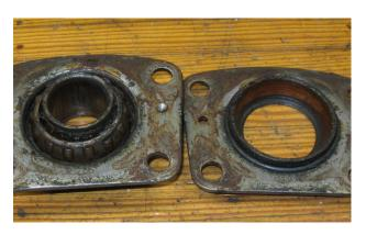
Fortunately, Clark's has all the internal parts to properly restore these to good working order, including new bearing cartridges. You do need the outer housings and inner shields, I was lucky enough to get the shields from John Sweet.
