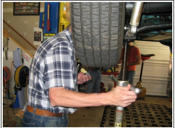
Frank multi-tasking a doughnut and cranking down the Underhoist support stand after tightening the stabilizing rod bracket to trans mount bolts.
