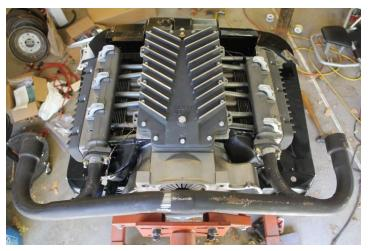
I like this picture showing that the pipes are adjustable left to right to allow for the heads being milled or not. Interested? Reply and ask questions for Art. arthooper@yahoo.com
