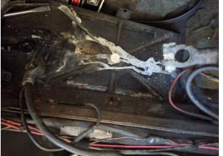
For a while, I have been meaning to clean my battery cables in the Corsa. I read that when starting the car, if the starter doesn't engage at times it could be corroded cables. I decided that it was time and I am glad I did. The positive cable was covered in corrosion. While that was bad, when I went to remove it from the battery the positive post rotated. Then I noticed acid streaks on the battery pan. It was a mess and I believe I got to it before I had an issue out on the road.
