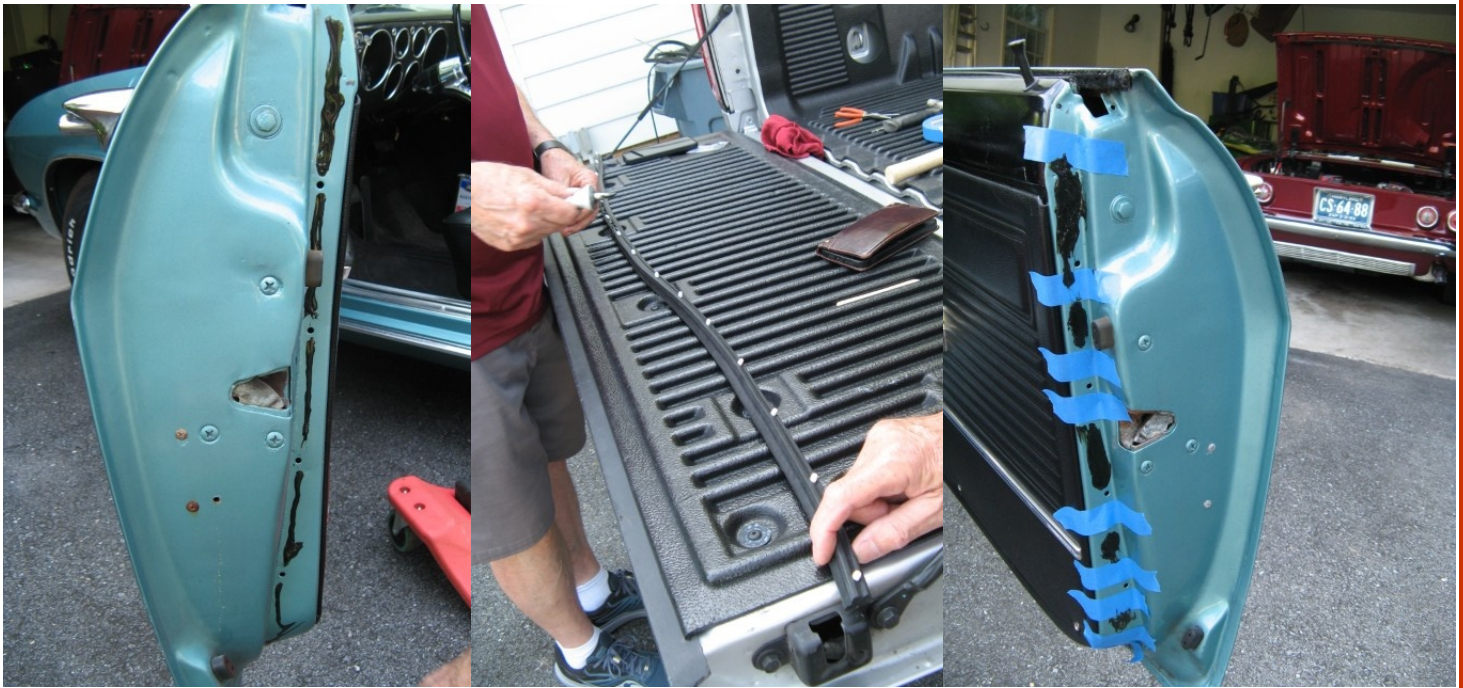
Put on the 3M glue and let it set a while on both door and seal. Start install by door lock up to front.
