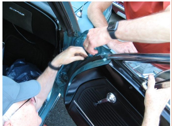
Put on the 3M glue and let it set a while on both door and seal. Start install by door lock up to front.
