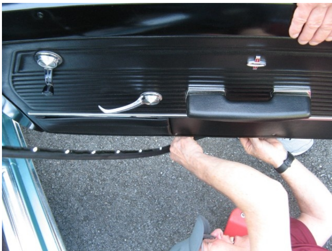
Put on the 3M glue and let it set a while on both door and seal. Start install by door lock up to front.
