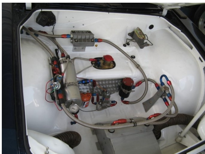
Fuel cell located where original tank was.
