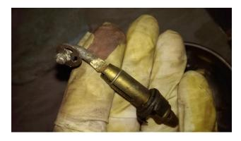
Removing it was easy. It literally fell off the pump. But how does one install the new rubber plunger. Bryan came to the rescue again. He mentioned that some people use a ball point pen end. I did exactly that and the rubber plunger slid on easily.
