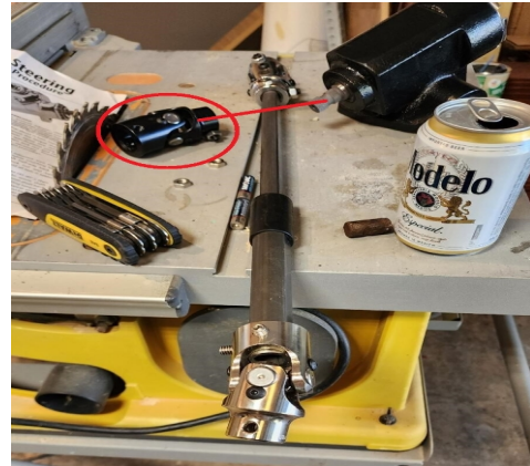
Circled joint is correct for box connection. Other two are wrong. Beer is right.
