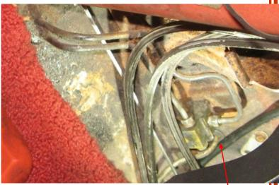
In this picture you can just see the new route taken for rear brake line to the front MC reservoir.
