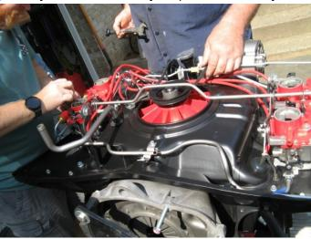
After a few weak cranks we ended up using TWO sets of jumper cables and jumped Jimmy's battery in his running Corvair to the engine and we had enough power then, and got the engine RUNNING.
