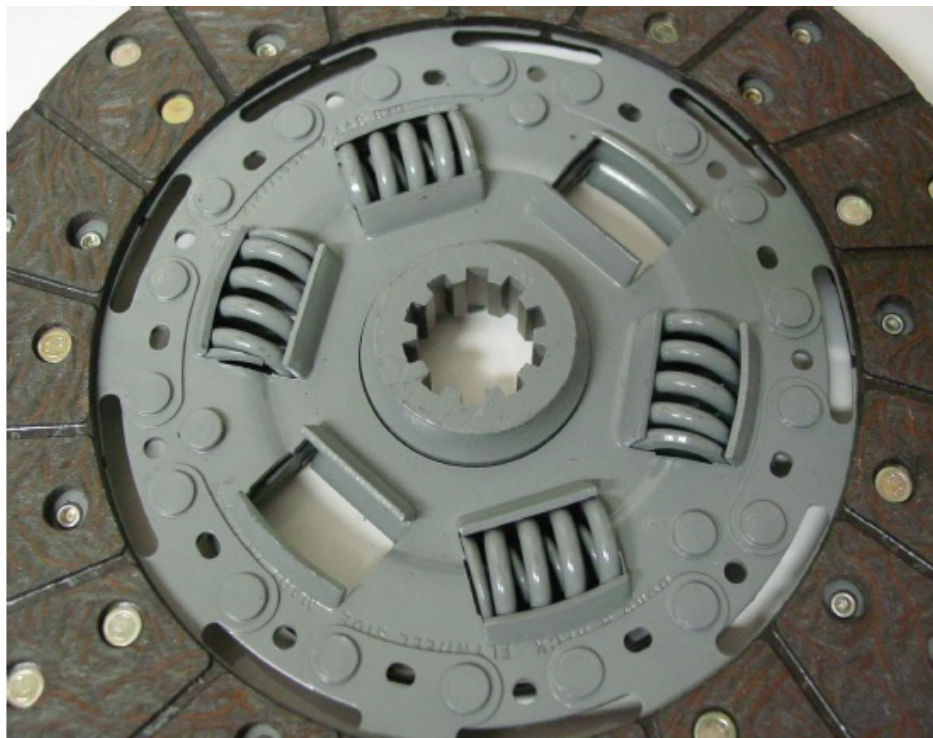
Above is pictured a Vega disc with damper springs and the center flywheel hub machined to clear the flywheel reinforcement on a Corvair.
