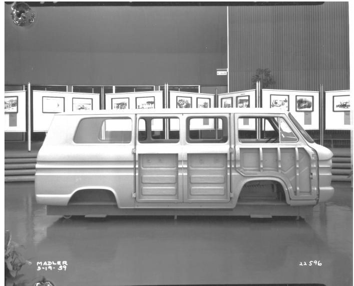
GM Photo of a wooden body buck of a Greenbrier van. If you'll notice in the background are images of renderings featuring some of the pre-production FC vans and pickups
