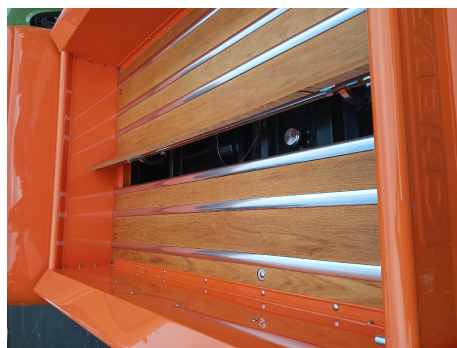
An innovative way to show one's underside - make part of the bed liftable to show the workings.
