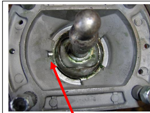
Lower seat raised key in base protrusion slot.
