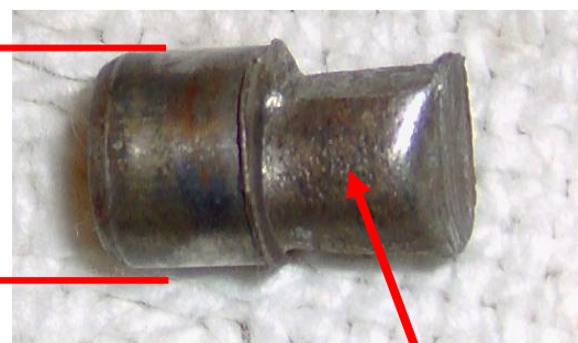
Old pin worn down by shifter lever
