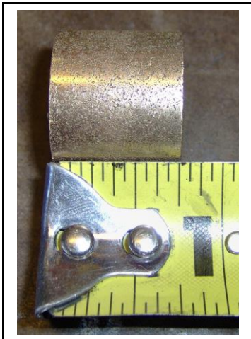
Example of brass or bronze bushing fitted inside outer tube.
