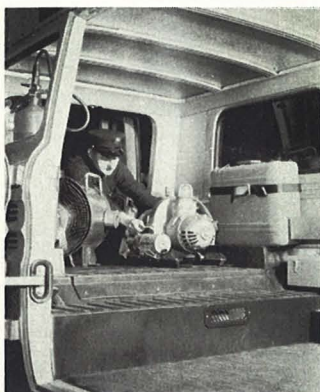
Portable generator, which powers a smoke exhaust fan, is placed in wagon by fireman Cyril Gunther. Masks worn by the "smoke eaters" are stored in kit under window.
