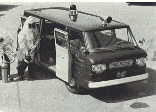
Fire-fighters wearing metallic, heat-resistant suits test extinguishers. Other emergency equipment carried by the Greenbrier includes a resuscitator, oxygen bottles, tarpaulin, blankets, heat-deflecting masks and gloves, and grappling and drag hooks.
