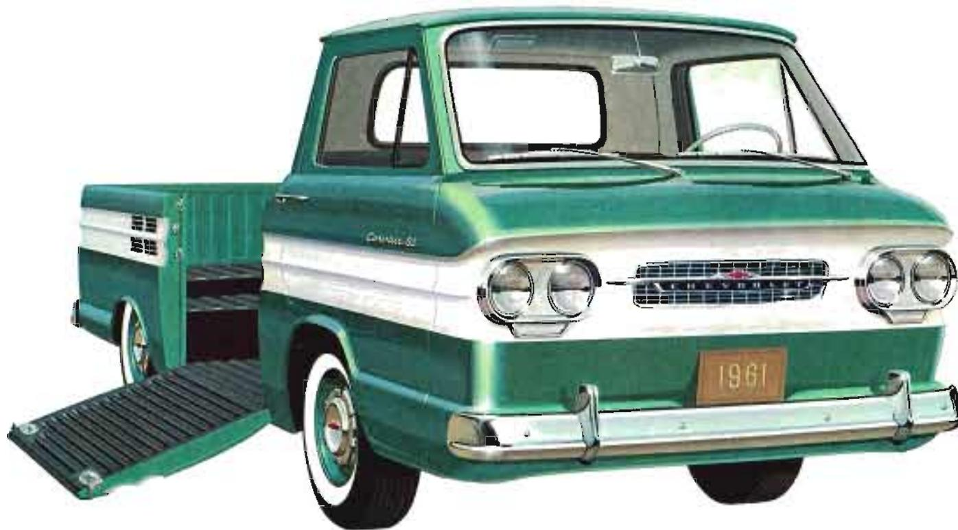
Here's something new and exclusive in pickups—*cargo-handling ease without precedent in the field!* A rugged-built cargo ramp swings down flush with the floor of the deep-well load compartment, leaving a gateway nearly four feet wide to get big loads in and out without lifting. With the floor less than 14 inches
