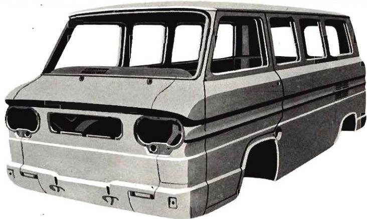
Unitized Body Construction of Corvair Greenbrier Sports Wagon.
