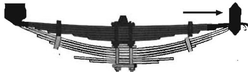
With heavier loads, the top leaf shortens, providing increased load support plus comfort. Engineering and on-the-road tests prove this to be the most ideal suspension ever offered on heavier-duty trucks.
