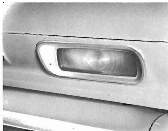
All light-duty models come equipped with new contrasting amber front parking and directional signal light lenses. These new lenses provide greater visibility, day or night.
