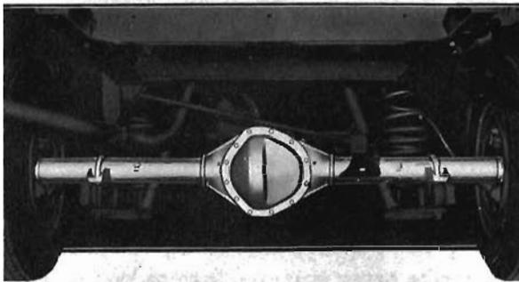
Stronger, quieter Salisbury-type rear axles for Two-Wheel-Drive Series 10 models also are new this year. Built-in ribs on the cast differential carriers, combined with steel tube axle shaft housings, provide new rear-end strength and durability.
