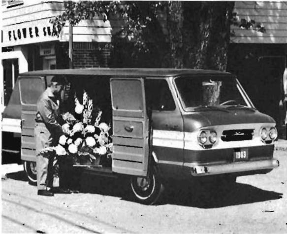
The Corvan has wide, low doors for easy loading and unloading. Left-hand doors are available for operations in crowded areas. Loading doors have new, strap-type, two-position door checks. Optional equipment for Corvans includes rear-door windows.
