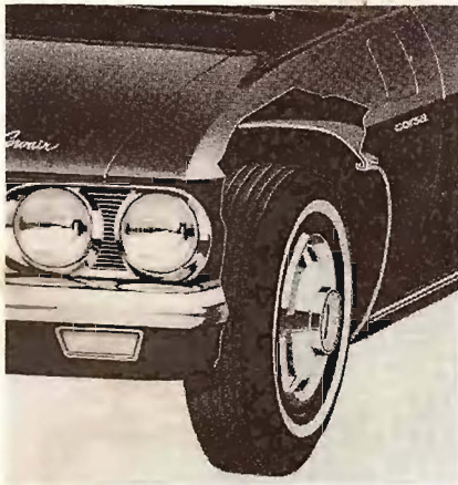
Protective inner skirts at both front and rear wheel openings help prevent corrosion damage to front fender and rear quarter sheet metal. Front fender skirt illustrated.
