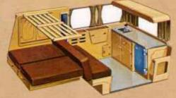
A custom unit that converts the Greenbrier into a mobile home. The unit includes wardrobe storage, counter-top with storage space below, ice chest, sink, water storage tank, vinyl floor, table, drawer storage, drapes and rods, rear storage space.
