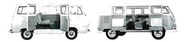
The Volkswagen Station Wagon is a true passenger vehicle. Its independent suspension imparts a comfortable ride with none of the left to right undulating motion and other disadvantages experienced with the rigid suspension of the Ford Station Bus. Nine people plus luggage comfortably fit in the VW, while only eight (with the two optional-extra rear seats) fit the Ford; seats, arm rests, heater-defroster, ash-trays, as well as quality workmanship are standard only on the VW Station Wagon.
