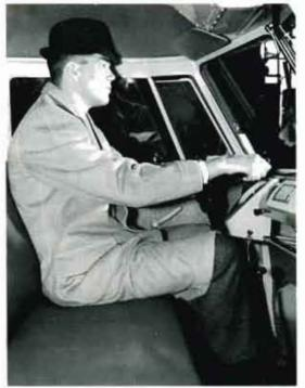
Headroom, a pain in the neck if you don't have it, as evidenced in the Ford picture, is clearly superior by two inches in the Volkswagen. The VW driver has plenty of room for his left arm compared to the cramped quarters of the Ford. A natural relaxed driving position is further aided in the VW by the almost horizontal steering wheel. The passenger seat is a \$35.40 extra on the Ford.
