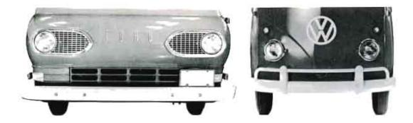
Ford Econoline vehicles do not come equipped with bumper guards and overriders, and they are not available as an option, while these items are standard equipment on the Volkswagen. Ford's combination parking lights and turn signals are placed low where they are vulnerable to damage and hard to see. The lower front door hinges stick out unprotected on the Ford. The VW hinges are shielded by the bumper guards.
