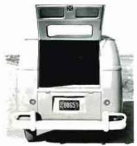
The Econoline's rear entry, 25 inches from the ground, offers somewhat easier loading from street level than the VW Panel, while dock-loading the VW Panel is relatively easier than on the Ford Van. Placement of the spare tire within the Ford Van necessitates unloading the truck to change a flat. In spite of similar loading space volume, the VW's payload capacity exceeds the Econoline Van by 930 lbs.
