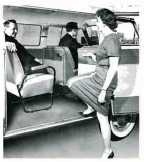
Just as the Ford Van is harder to load because of the five-inch higher floor line, so is entrance to the Ford Station Bus—especially for the ladies.
