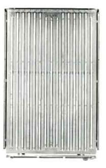
The VW Pick-up offers hinged sides that drop down, as well as the tailgate, converting it in seconds to a roomy flat-bed truck with 45 square feet of perfectly level floor space. The Econoline pickup bed, 17 inches shorter than the VW, is interrupted by two wheel housings and a spare tire. Access to the Ford bed is limited to the rear. Wooden runners, standard equipment on the VW Pick-up protect the truck bed.
