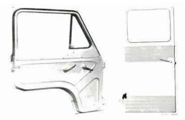
The Greenbrier's six doors resemble the one pictured above; they are lined with painted sheet metal and are heavy and tend to sag, easily dropping out of alignment. Volkswagen's doors are lined with leatherette, matching the other interior appointments, and notice how dark colors are utilized in areas subject to scuffing and handling. Poor fitting and sealing of the doors lets wind, rain, dirt and snow into the Corvair 95 passenger vehicle.
