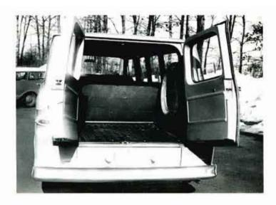
The Greenbrier, with none of these "deluxe" features, has a bare metal luggage compartment containing the spare tire and lined with the metal engine compartment lid which must be removed along with luggage to reach the engine.
