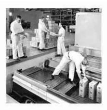
The Volkswagen is just as easily loaded or unloaded from sides or rear. The Chevrolet tailgate does not drop down vertically, making loading and unloading awkward, and preventing the vehicle from being backed up flush against a loading dock. Also note, that the VW Pick-up bed is much closer to the height of the standard loading dock, particularly convenient for farmers and tradesmen who regularly pick up and deliver at truck terminals.
