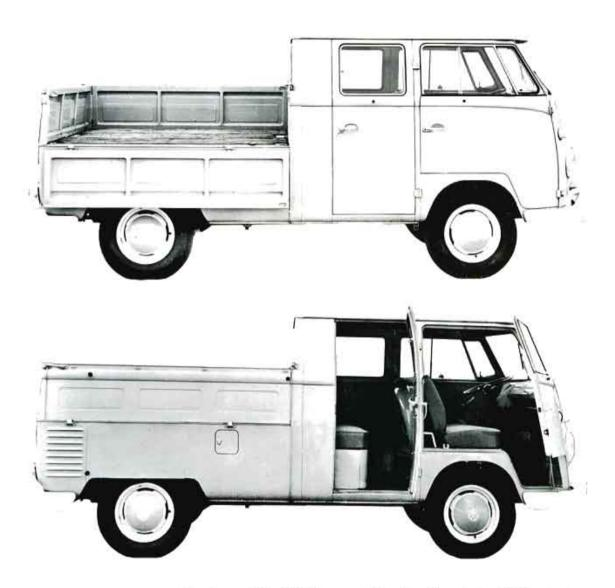
Here's a vehicle that the competition hasn't copied yet! There's room for six people and the flat loading platform, which is at loading dock level, has tail-gate and sides that drop vertically. Under the second bench seat is a built-in tool chest. With the second seat removed, it becomes a three-passenger pickup with 57 cubic feet of enclosed, lockable, weathertight cargo space—30 square feet of loading area in the rear.
