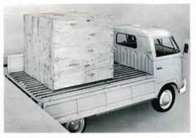
Bulky crates, difficult to load, will not sit flat in the Chevrolet Pickup. A load such as this necessitates an outside rear view mirror, standard equipment only on the VW Pick-up. Volkswagen's three hinged drop-sides permit easy loading of crates the size of the bed, 75.6 inches wide and 169.3 inches long. Rear access to the Chevrolet Pickup is limited to loads only 44¾ inches wide, and loads entering through the ramp opening are limited to 47½ inches wide.
