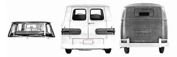
An annoyance feature on the Corvan is the rear windows, split by a door post that obstructs vision, making it difficult to see to the rear. Rear bumper guards and overriders are not available on the Corvan. Quality again—notice the difference in the way the Chevrolet doors fit; there is a minimum of space around the VW doors, while on the Corvan, space surrounding the doors permits snow, rain and wind to enter the vehicle.
