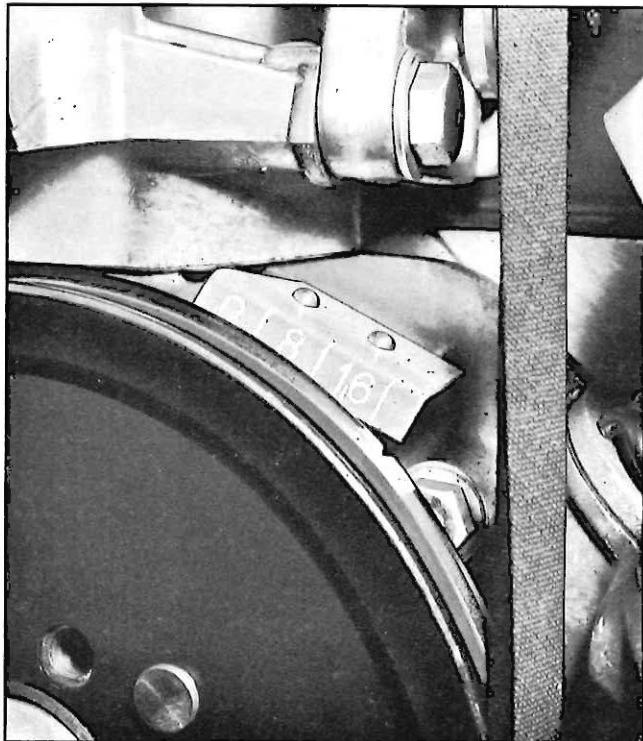
*Fig. 10 Ignition Timing Setting*
