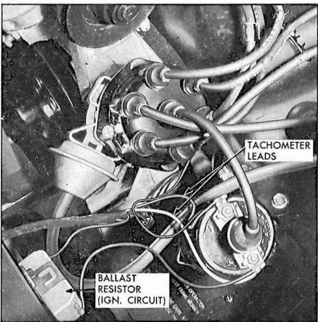
Fig. 44—Ignition and Electric Tachometer Wiring
