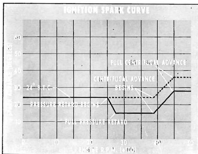
Fig. 42—Distributor Spark Curve
