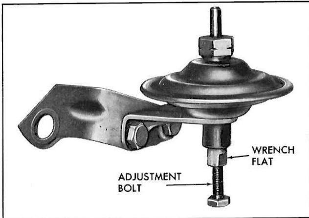
Fig. 6—Throttle Return Check Valve
