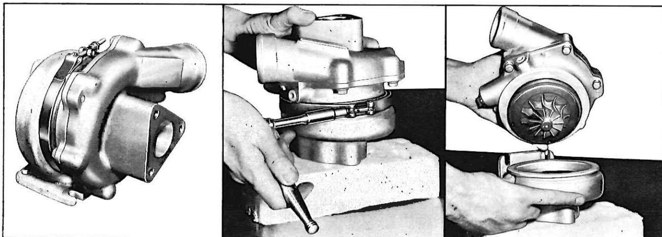
Fig. 37—Removal of the Turbine Housing for Installation of Replacement Supercharger
