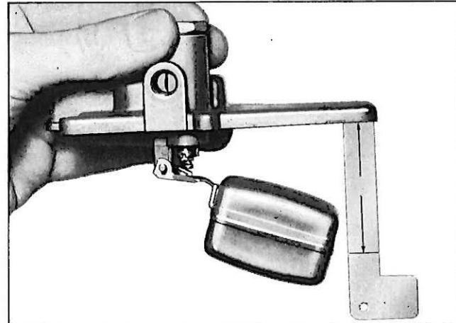
Fig. 9—Measuring Float Drop
