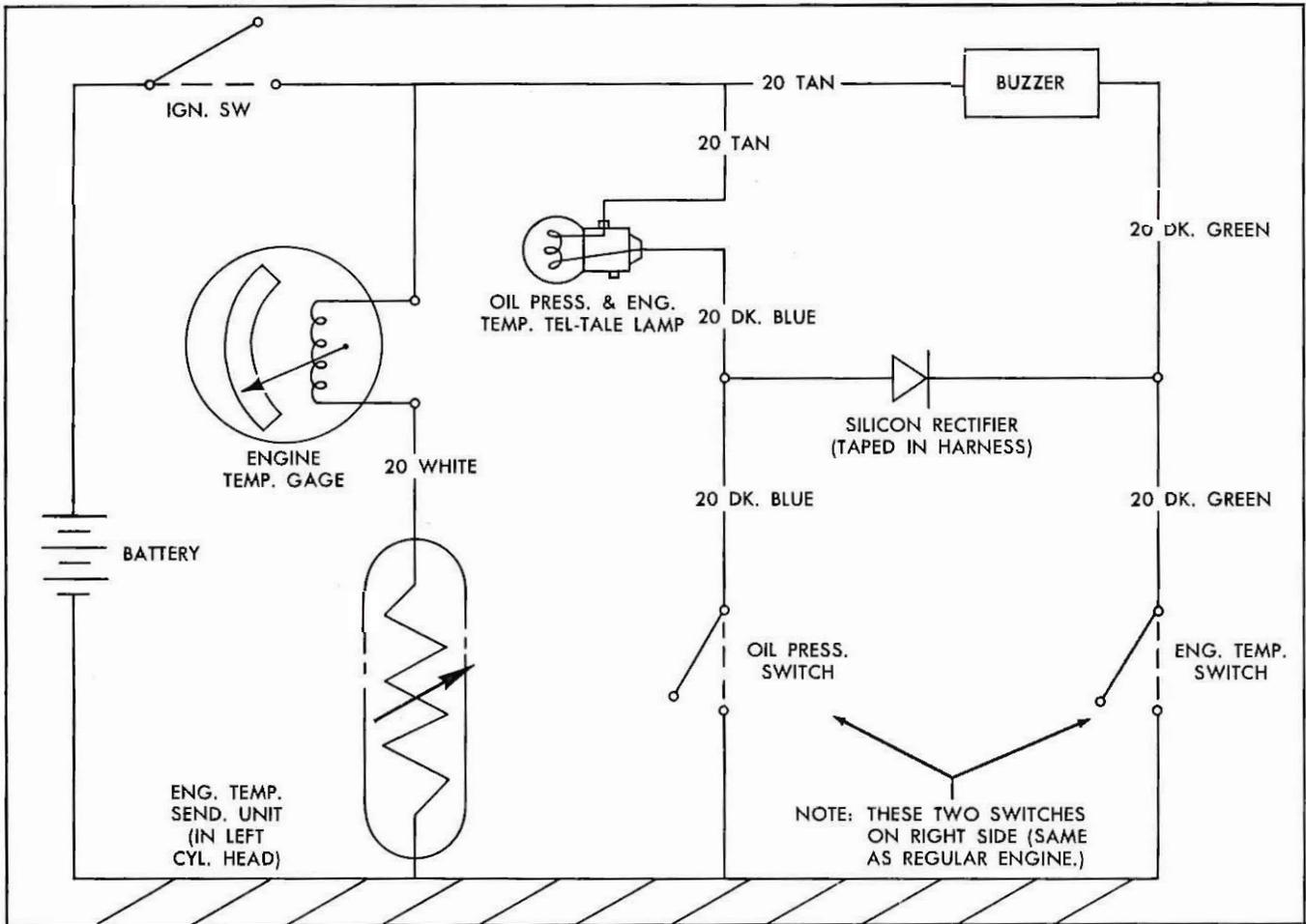
Fig. 45—Oil Pressure and Engine Temperature Tell-tale Lamp, Temperature Gauge and Warning Buzzer Wiring
