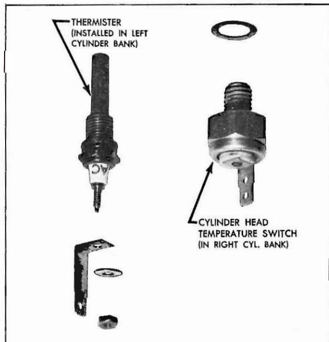
Fig. 46—Cylinder Head Temperature Sensing Units
