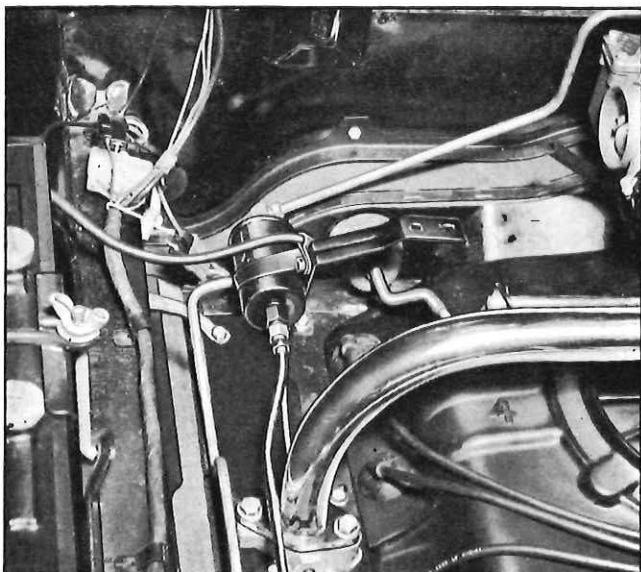
Fig. 4—Fuel Filter Installed
