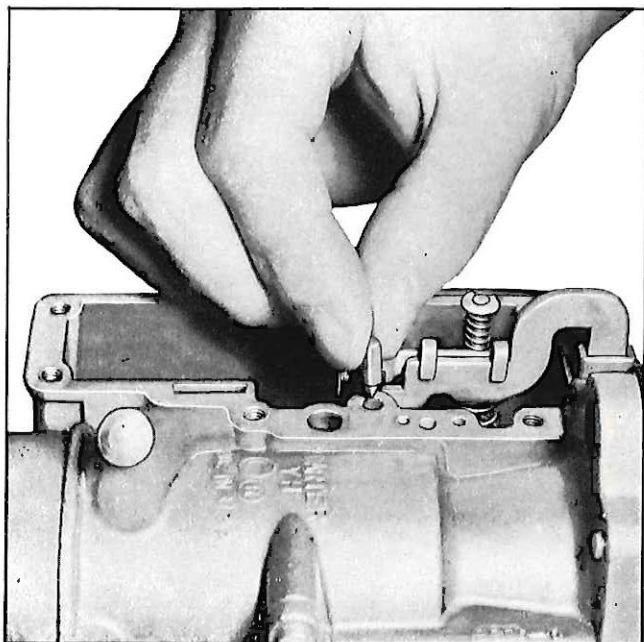
*Fig. 18—Install Pump Discharge Needle*
