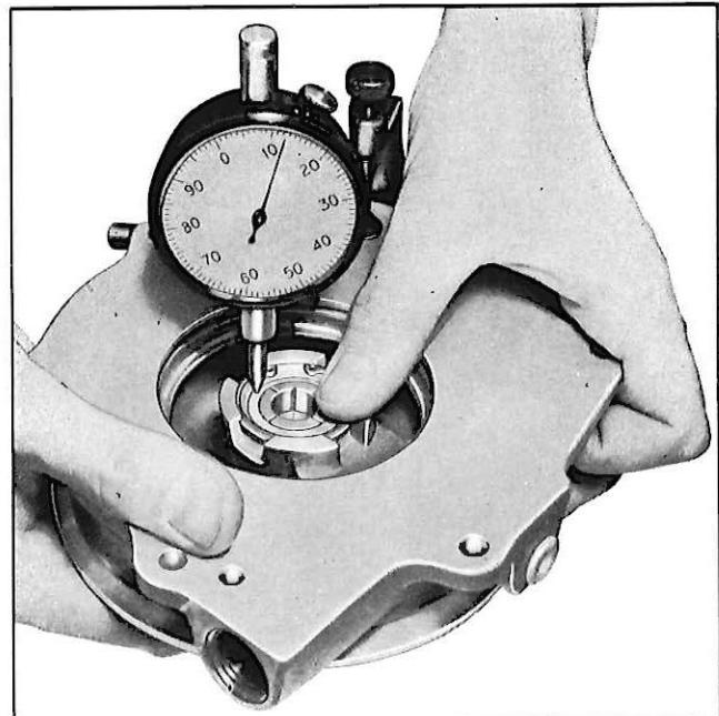
*Fig. 28—Gauging Bearing-to-Housing End Play*
