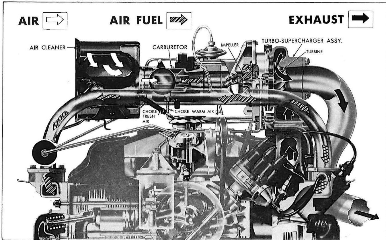
Fig. 1—Turbo-Supercharger Operation on Corvair Engine
