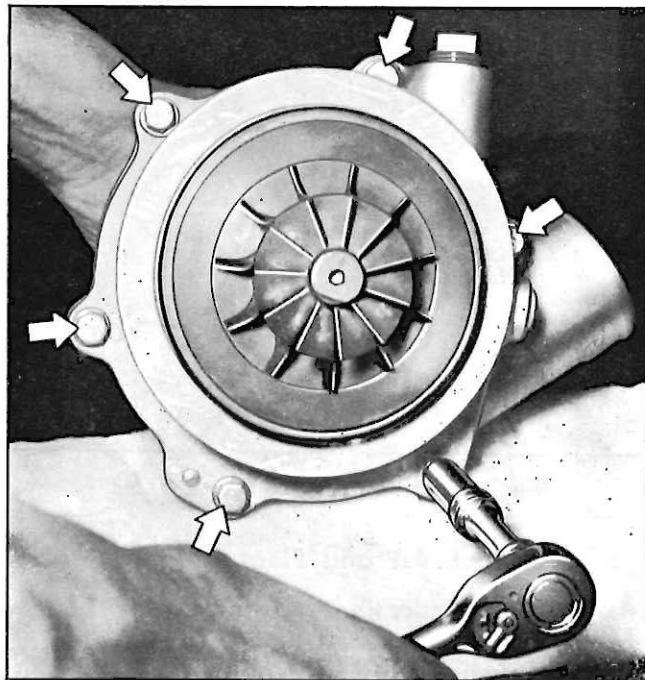
*Fig. 11—Compressor Housing Retaining Bolts*
