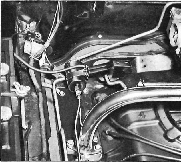
Fig. 4—Fuel Filter Installed
