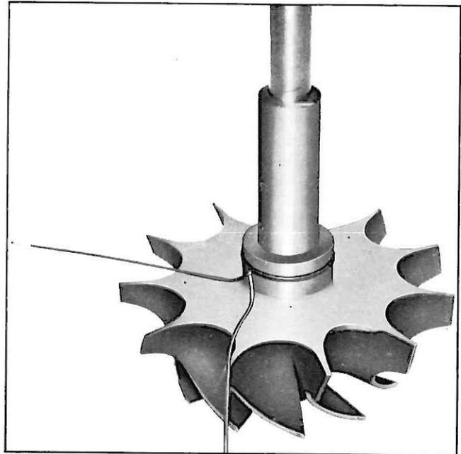
Fig. 31—Ring Compressed, Using Tag Wire
