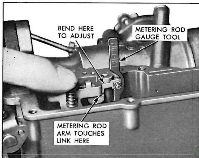
Fig. 17—Adjust Metering Rod Arm
