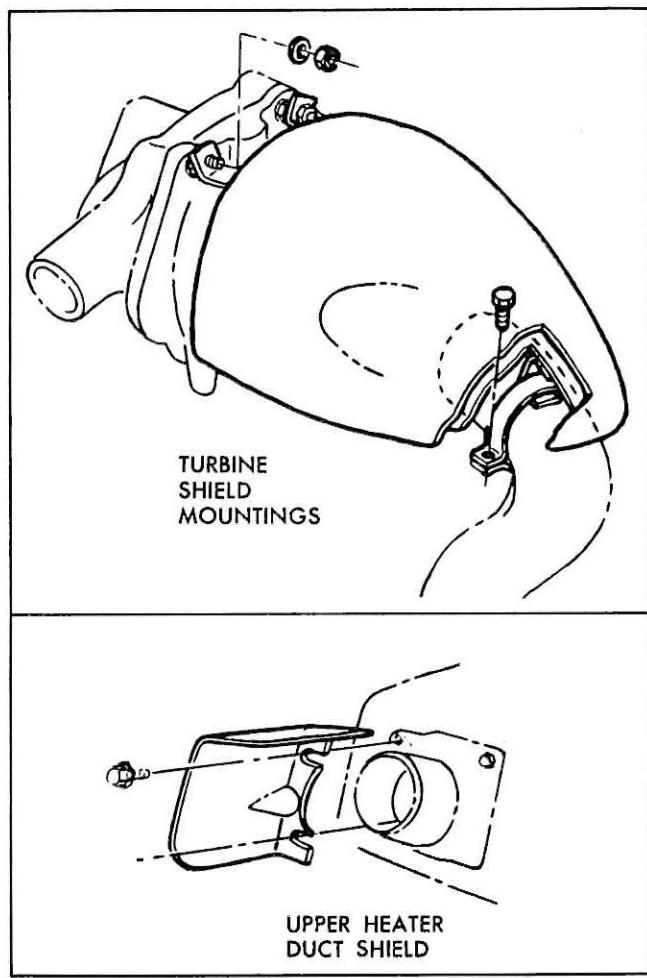
Fig. 39—Turbine Exhaust Heat Shields
