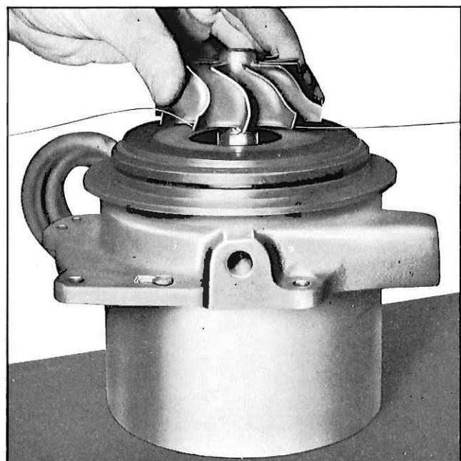
*Fig. 33—Installation of Turbine Wheel and Shaft*
