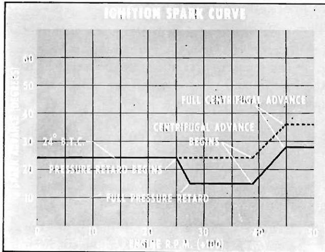
Fig. 42—Distributor Spark Curve
