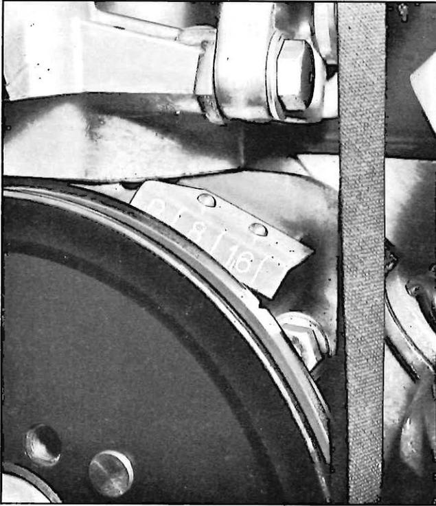
*Fig. 10 Ignition Timing Setting*
