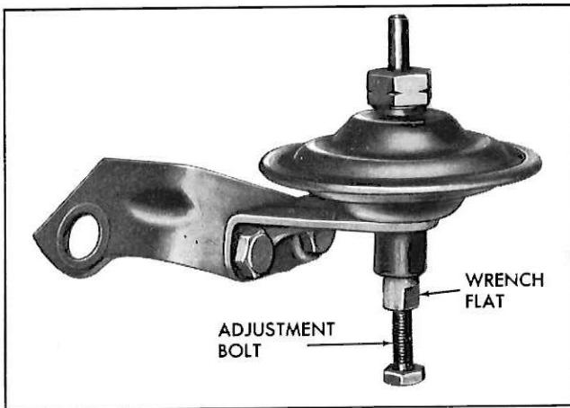
Fig. 6—Throttle Return Check Valve
