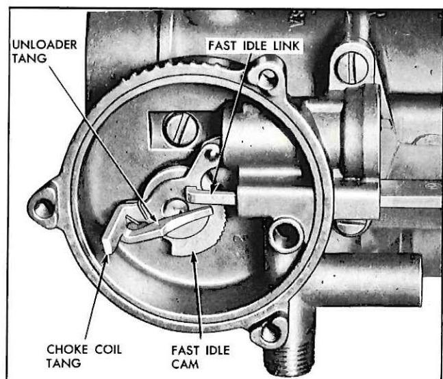
*Fig. 19—Choke Housing and Fast Idle Linkage*
