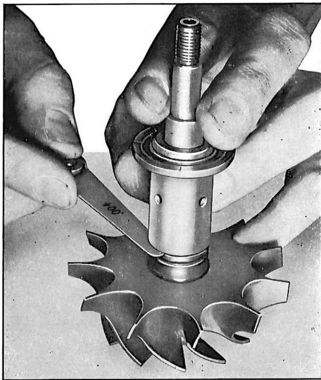
*Fig. 27—Measuring Bearing-to-Shaft End Play*
