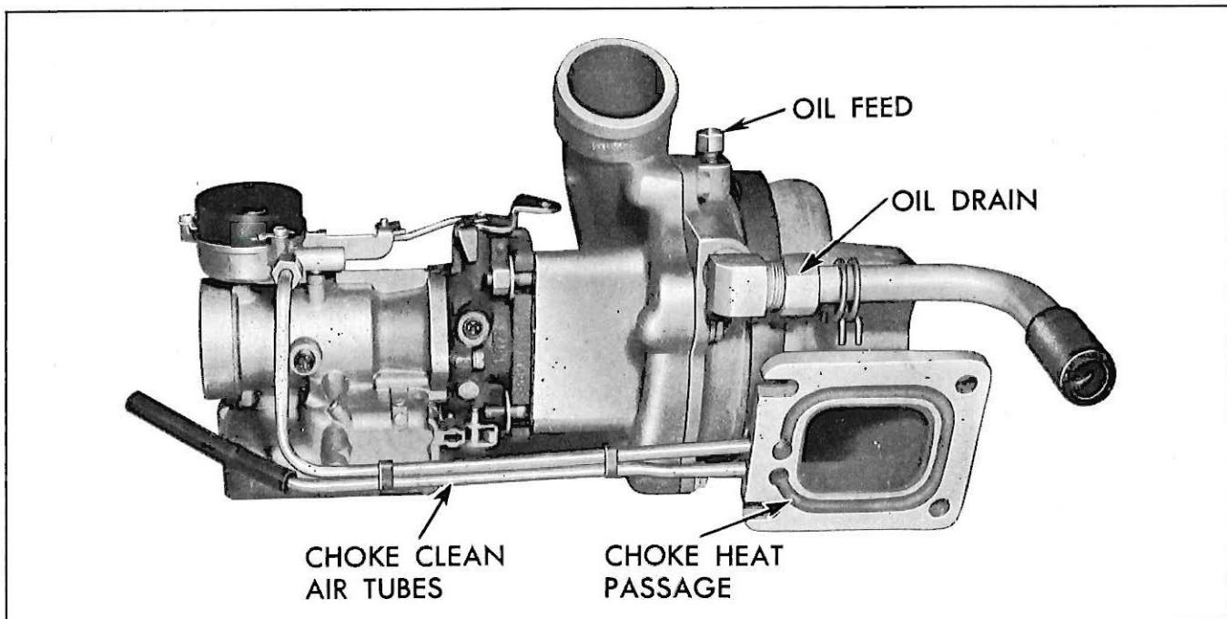
Fig. 38—Carburetor Fittings and Passages
