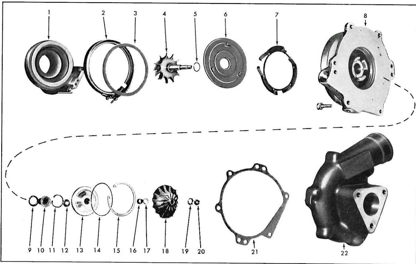
Fig. 26—Turbo-Supercharger (Exploded View)
