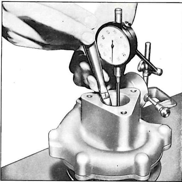
Fig. 29—Gauging Impeller-to-Housing Clearance
