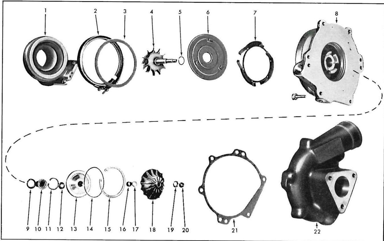
Fig. 26—Turbo-Supercharger (Exploded View)
