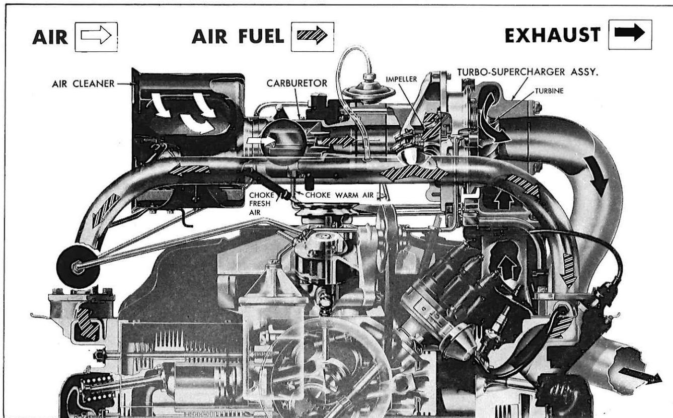
Fig. 1—Turbo-Supercharger Operation on Corvair Engine
