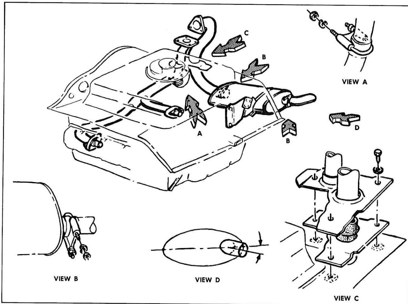
Fig. 40—Exhaust System Components
