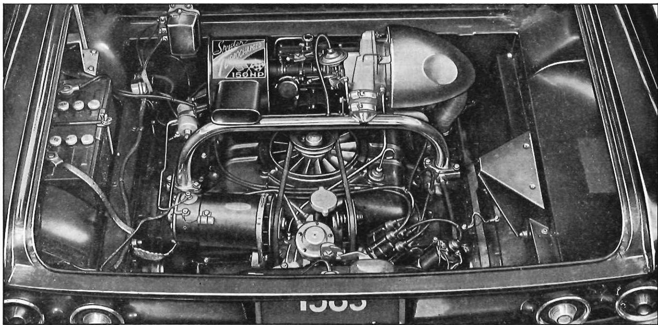
Fig. 2—Turbocharged Engine Installed
