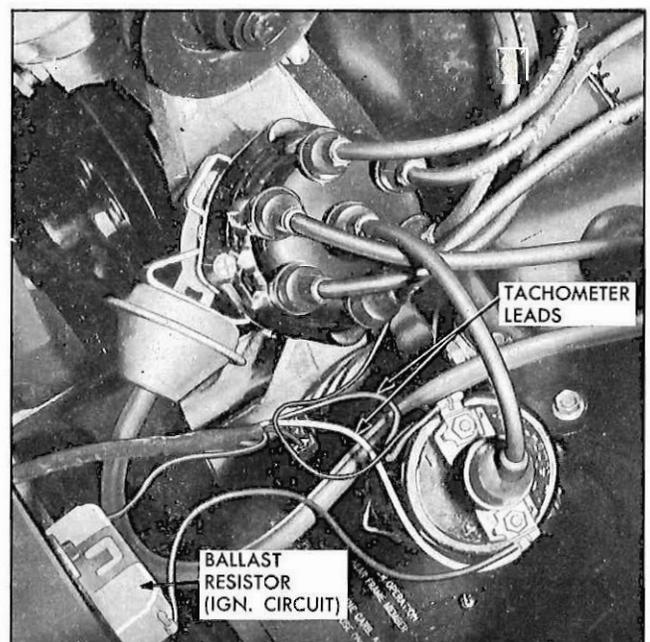
Fig. 44—Ignition and Electric Tachometer Wiring
