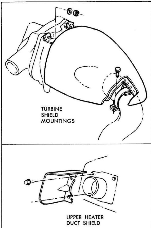
Fig. 39—Turbine Exhaust Heat Shields
