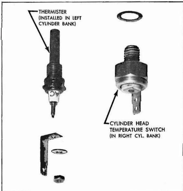
Fig. 46—Cylinder Head Temperature Sensing Units
