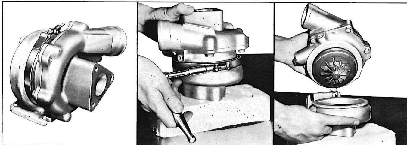
Fig. 37—Removal of the Turbine Housing for Installation of Replacement Supercharger
