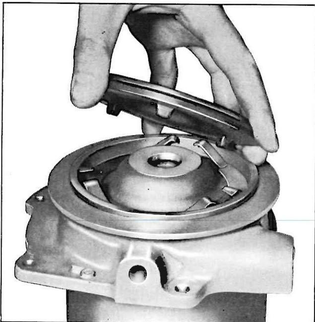
Fig. 30—Heat Shield Spring Ring Installation
