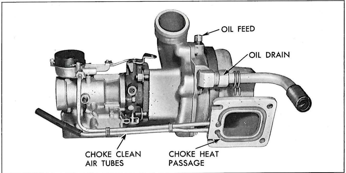
Fig. 38—Carburetor Fittings and Passages
