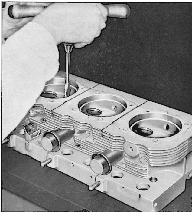
Fig. 2—Reaming Cylinder Head Valve Guide Bore
