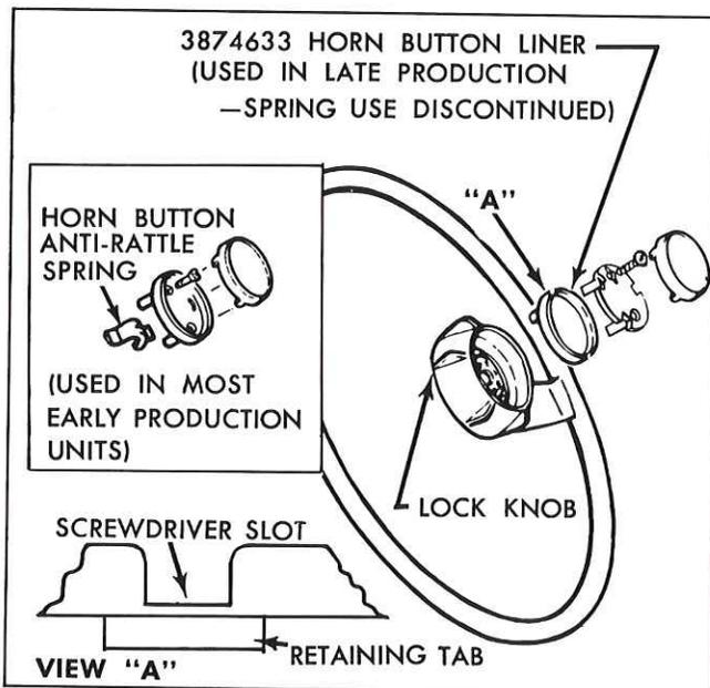
Fig. 8—Telescoping Steering Wheel Horn Button Liner
