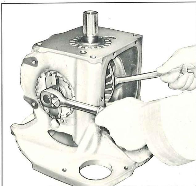
Fig. 7—Adjusting Ring Gear To Pinion
