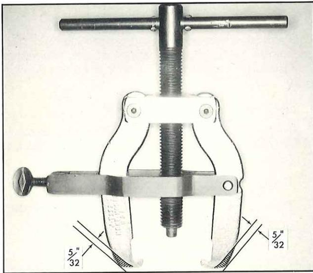
Fig. 6—Bearing Puller J-7112 Modification
