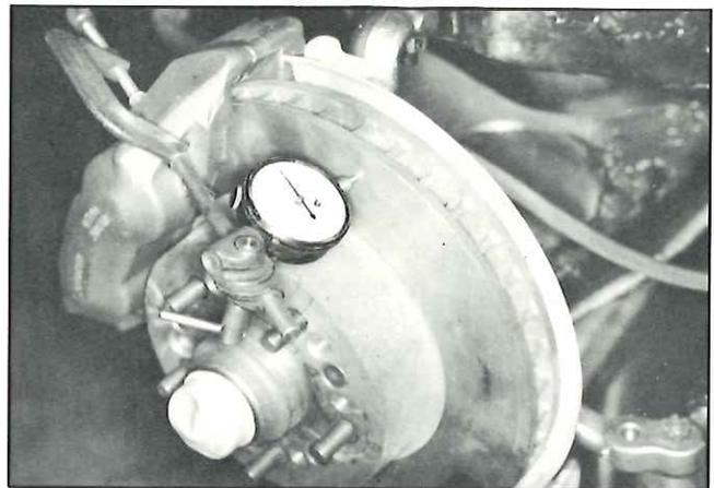
Fig. 11—Dial Indicating Disc Runout
