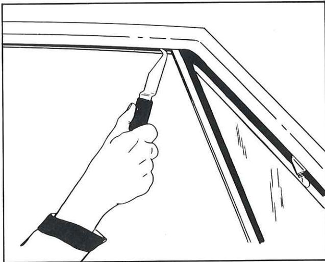
Fig. 1—Door Window Glass Run Channel Removal
