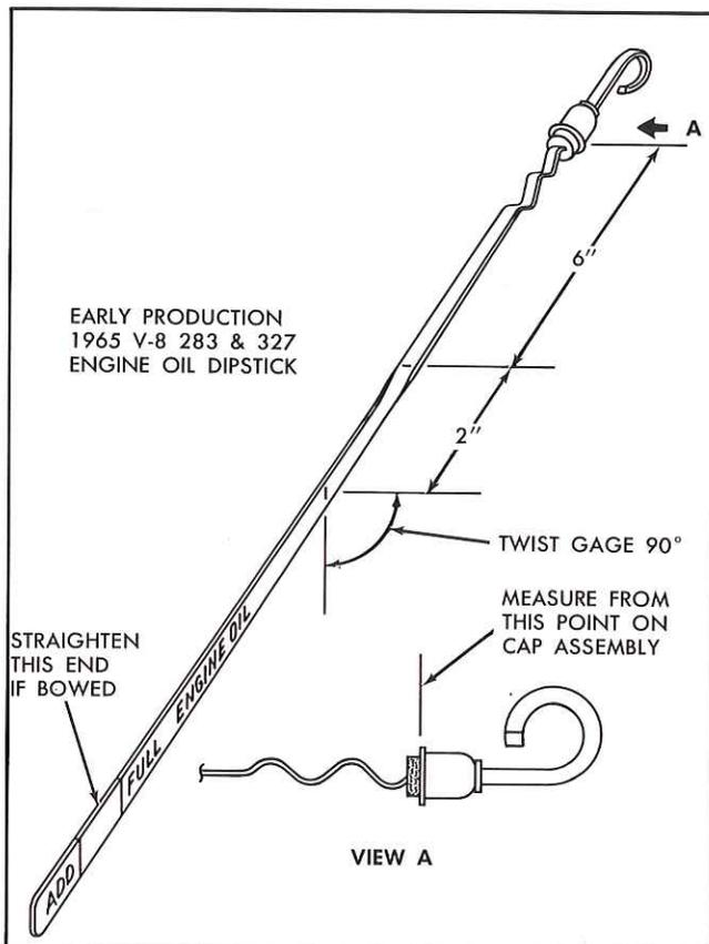
Fig. 4—V-8 (283 or 327 cu. in.) Engine Dip Stick Modification
