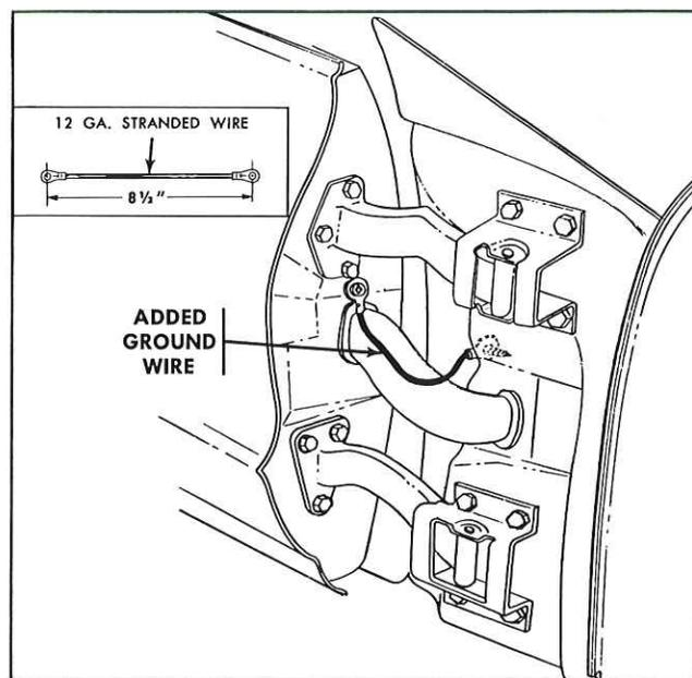
Fig. 9—Power Window Ground Wire Added
