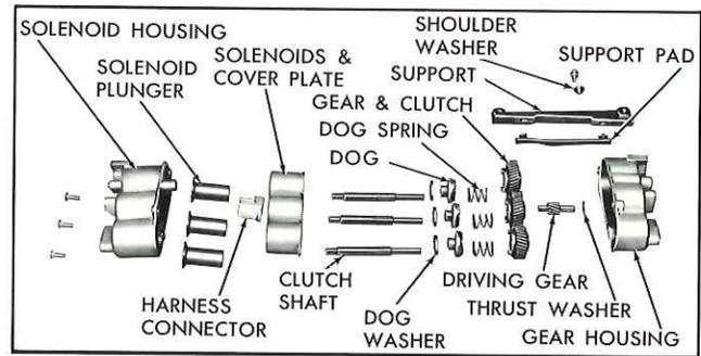
Fig. 2—Six-Way Transmission Components
