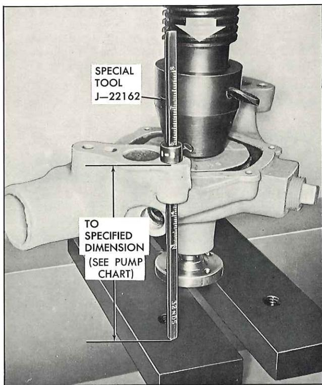
Fig. 15—Fan Hub Locating Tool
