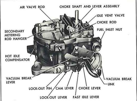
Fig. 2—Rochester Quadra-Jet Carburetor—Model 4MV
