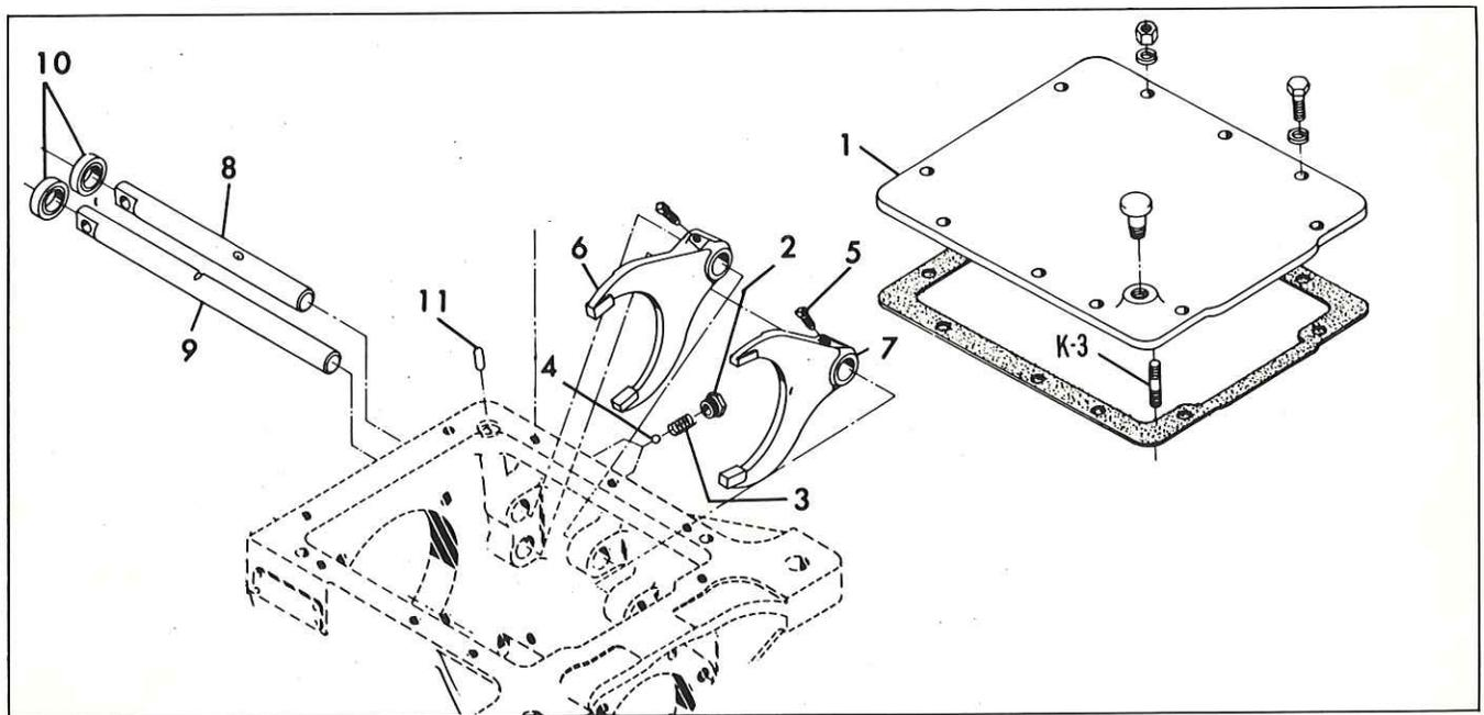
Fig. 7—Auxiliary Transmission Shift Controls and Cover
