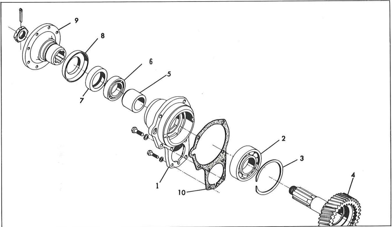
Fig. 11—Main Drive Gear and Bearing Details
