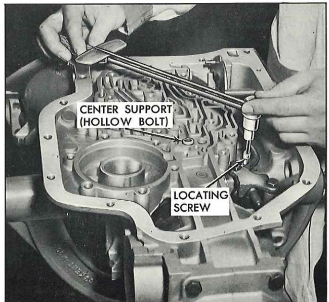
Fig. 13—Locating and Locking Case Center Support
