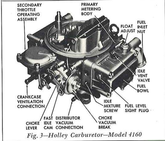
Fig. 3—Holley Carburetor—Model 4160
