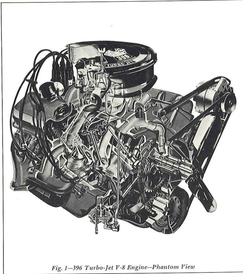
Fig. 1—396 Turbo-Jet V-8 Engine—Phantom View
