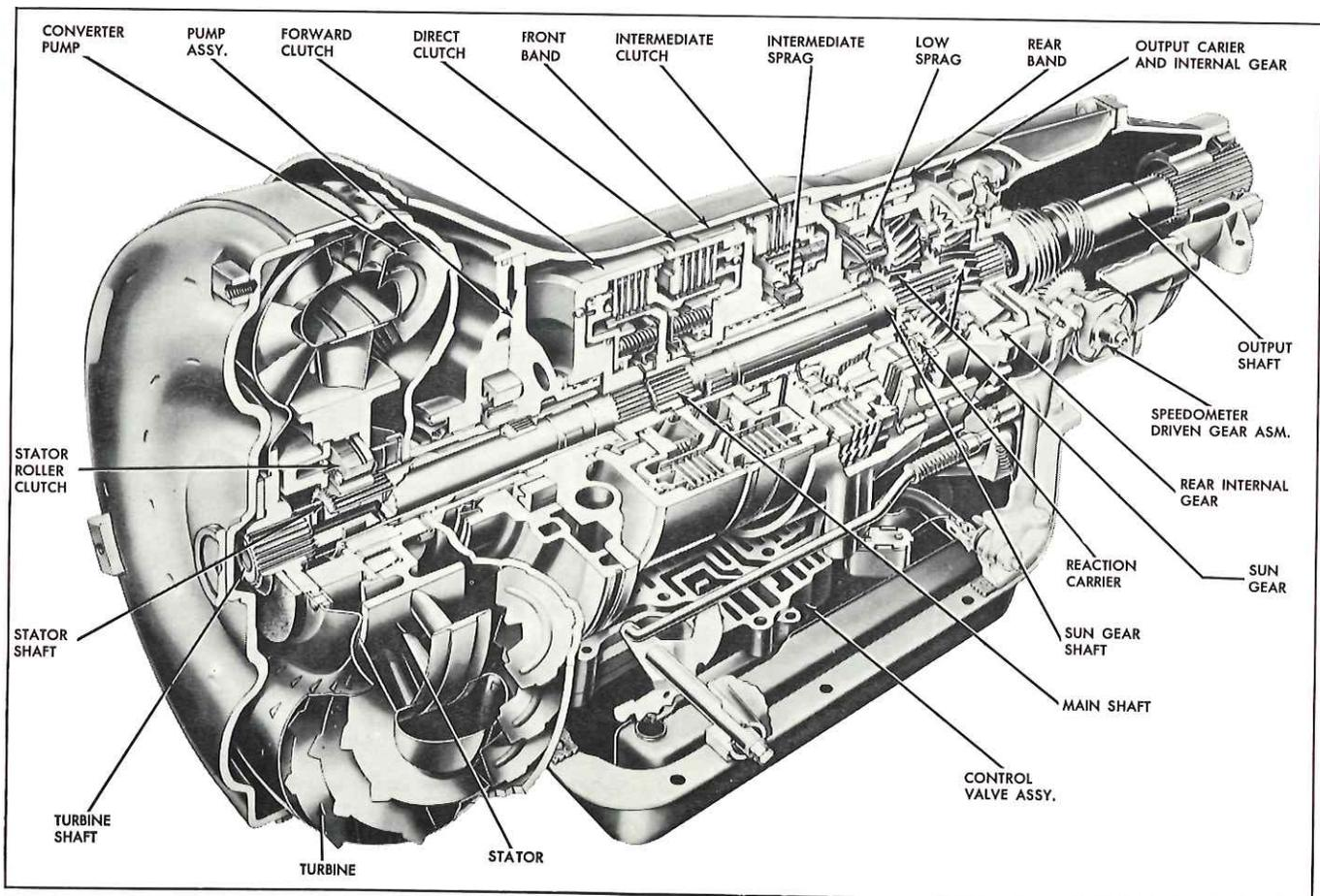
Fig. 5—Turbo Hydra-Matic 3-Speed Automatic Transmission
