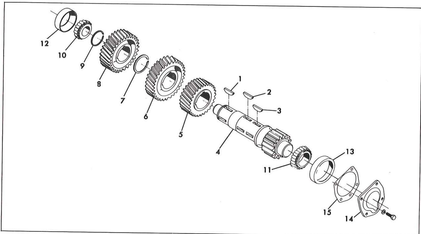
Fig. 9—Countershaft with Gears and Bearings
