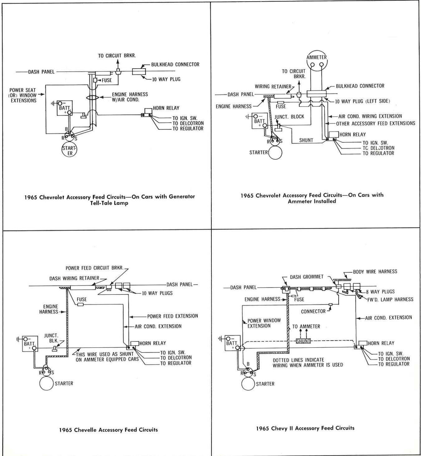
Fig. 6—Power Feed Wiring for Various Electrical Accessories
