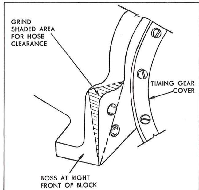
Fig. 14—Cylinder Block Rework for Hose Clearance
