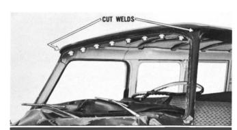
The front roof trim panel was removed to provide access to the 8 bolts which hold the windshield header to the inner roof rail. Welds were cut to separate the cowl pillars from the roof rails.
