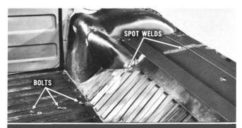
— through the dropped floor panel and the welds across the seat riser are accessible from inside the body. The damage in the kickup panel will be straightened after strain on it from the side rail has been relieved.
