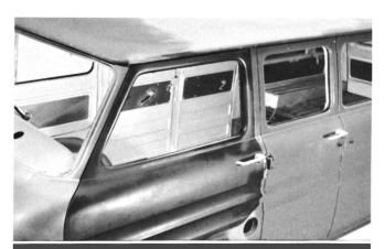
The roof panel was then metal-finished and primed.
