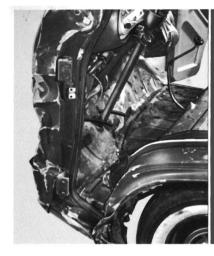
— the toe panel, front floor panel, the left rocker panel assembly, steering column and instrument panel are all damaged extensively. The installation of new parts and assemblies is the only practical and profitable repair procedure.
