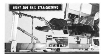
The frame machine was set up to concentrate tension on the front buckle. Attachment to the front end of the right side rail was made by a brazed-on heavy metal strip, clamp and chain. Heat was necessary to aid straightening.
