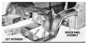
The left outrigger (clutch and brake pedal support) and the rocker panel assembly were clamped in place and tack-welded. The installation of these parts was necessary to establish a reference point for measuring the distance between the rocker panel and roof.
