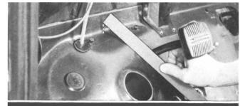
On the interior, the toe panel was forced upward, forming a bulge in the area surrounding the steering gear column opening. Both the steering gear mast jacket and worm shaft were bent. There was no indication of side rail misalignment.
