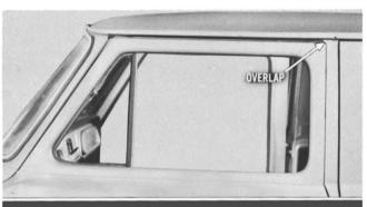
The left front cowl hinge pillar was pushed slightly rearward at the belt line, causing the door to drop and overlap at the lock pillar. This completes the inspection of damage conditions.
