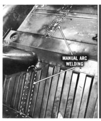
Manual arc welding is recommended to join the floor panel to the heavy-gauge side rails, because of the holes left by the spot-weld cutter. If gas welding is used, the flange of the side rail should be preheated from the underside.
