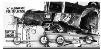
— by adding another bracket at the forward end of the side rail. An allowance of '4" was added to the datum line height setting of the bracket and then clamped in place. Correct alignment is shown by a lengthwise bar touching each of the brackets and centerline gauges.
