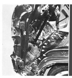
The toe panel was separated from the front floor panel by removing 11 bolts extending across the joint.
