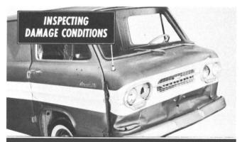
On the exterior, the outer cowl panel above the bumper, the area over the left headlight and the right door are dented.
