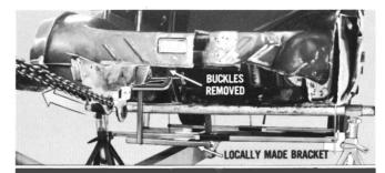
Attachment of the frame machine was shifted to the lower flange of the right side rail to apply tension to the buckles under the seat riser. Heat was also used. A locally made bracket was set to datum height and then clamped to the side rail at the front suspension attachment. The bracket—
