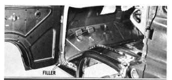
After the brake and clutch pedals were installed, the left outrigger was shifted slightly to permit proper pedal movement in the toe panel openings. The outrigger and door filler reinforcements were then welded in position. All other welding was then completed. Bolts to the header rail and toe panel were installed.
