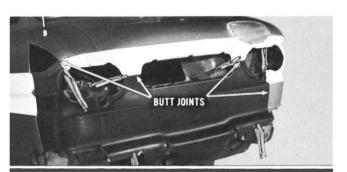
The new cowl panel unit was then placed on the cowl and temporarily clamped in position. Minor corrections to provide butt joining were then made to the new panel by shifting the panel slightly as needed and trimming the metal where necessary.
