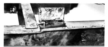
A door was cut in the upper flange of the right side rail. Heat and a heavy curved body spoon were used to force the minor buckles outward from inside the box section. This permitted final straightening with hand tools. Gas welding was used in closing the door and repairing the torn section.
