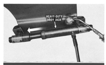
Heat was applied to the sharp buckle as the dent was pulled out by extending the body jack.
