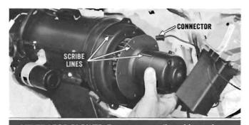
VENTILATOR BLOWER: To remove ventilator blower from heater, separate connector at motor terminal. Scribe a line across blower housing, motor mounting plate, and motor. Remove four retaining screws and remove motor and fan assembly.
