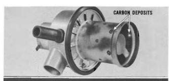
If the carbon build-up is uneven, carbon deposits clog or partially clog the air holes, or small areas of the mixer cup are excessively burned, the burner has been operating with an insufficient supply of combustion air, a one-sided fuel spray; or there has been fuel leakage inside burner casting.
