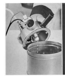
Have someone disconnect live electrical lead at car. Fuel spray should stop. NOTE:
