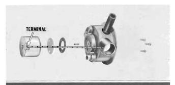
NOTE: When installing solenoid cup assembly, use a new gasket between sealing disc and burner housing. Make sure coil terminal is approximately in line with burner air inlet opening. Retest burner assembly for correct spray pattern and complete fuel shut-off.
