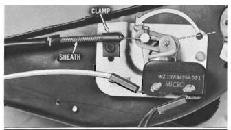
Move HEAT control lever to full "up" position. Make sure there is no interference with cable sheath when thermostat tension lever is in full counterclockwise position.
