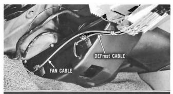
The DEFrost and FAN control cables have "eyed" ends at air distributor. The only adjustment possible to obtain full travel of either of these controls is by shifting the cable sheath in its retaining clamps.
