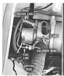
Remove the burner assembly from the car as follows: Disconnect the spark plug ground wire and fuel solenoid wire. Separate high tension cable from spark plua. Disconnect fuel line to burner. Loosen clamp securing combustion blowerthoserto casting.
