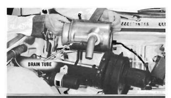
Disconnect the drain hose from the heat exchanger drain tube. Shift the lower heater case towards the front of the car. Remove heat exchanger.
