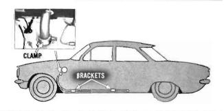
EXHAUST TUBE: To replace the exhaust tube, loosen the clamp which secures the exhaust tube to the heat exchanger outlet tube. Remove the bolts which secure the exhaust tube to mounting brackets on the car underbody.
