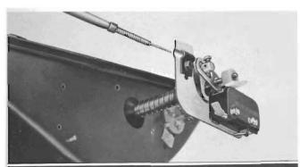
Disconnect HEAT control cable from thermostat and remove screws which secure thermostat to air distributor. Install new thermostat and adjust cable as shown previously.
