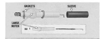
Before installing the spark plug remove the rubber sleeve and carefully inspect the porcelain for cracks. Inspect for badly burned electrode. If necessary, remove the electrode from the porcelain and clean electrode with emery cloth. When reassembling spark plug, the electrode should point away from the large notch in porcelain. Examine rubber sleeve and the two plug gaskets and replace if necessary.
