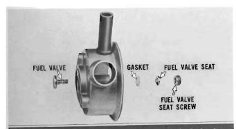
NOTE: It is not normally necessary to remove the fuel valve seat screw, valve seat and gasket from the burner housing. If these parts are removed for any reason, the fuel valve nylon gasket must be replaced.
