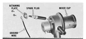
Remove two screws which secure the spark plug retaining plate and ground wire to the burner housing. Remove spark plug. Inspect spark plug electrode, and the ground electrode attached inside the mixer cup. If electrodes are badly burned, both the spark plug and the mixer cup must be replaced.
