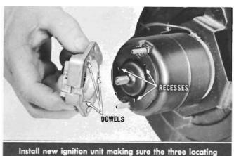
Install new ignition unit making sure the three locating dowels enter the recesses in motor end plate.
