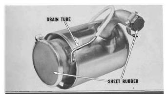
To test heat exchanger, block burner inlet and exhaust outlet openings with sheet rubber held in place with clamps. Connect rubber hose to drain tube.
