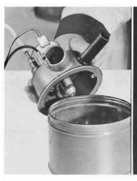
Run a lead from the fuel solenoid terminal to some point where it can be connected to a convenient live terminal on the car. Do not connect lead at this time.) Connect a ground lead between the car and the burner housing. The electrical lead should be connected and disconnected at the car because of the hazard of arcing at the burner assembly and possible ignition of gasoline.
