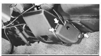
HEATER CONTROLS: The adjustment of the HEAT control cable is very important. To check adjustment, remove screws from cover on right side of air distributor. Remove cover.
