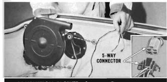
COMBUSTION BLOWER: Separate 5-way connector located on heater. Remove black and white wires leading to blower from the connector. Free these wires from clips. Disconnect outlet hose from blower. Remove the three attaching bolts and remove blower from car.
