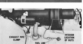
Disconnect exhaust pipe clamp and fuel line connections. To obtain clearance for removing heat exchanger remove two nuts holding ventilator blower case in place. (These two nuts are in the passenger compartment. One is located in the air distributor.)
