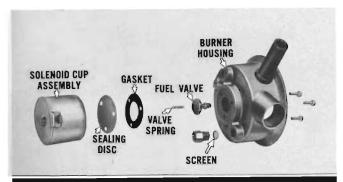
Remove fuel inlet fitting and screen. Remove three screws securing solenoid cup assembly to burner housing. Separate solenoid cup assembly, sealing disc, gasket, fuel valve spring and fuel valve from burner housing.
