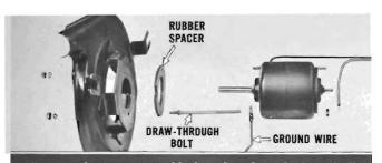
Remove the two nuts and lockwashers from the inner half of the blower case. Separate motor and rubber spacer. When reassembling, attach the ground wire between the draw-through bolt and the motor housing. NOTE: Replacement motors have two wires. The black wire leads into the motor case. The white wire is an extra ignition unit wire and should be discarded.
