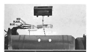
When replacing Purge Switch, be sure to solder wires to new switch as shown. Note that switch cover is secured by two spring tangs in front and one screw at rear.
