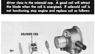
Remove solenoid coil cover screw and cover. Install new solenoid coil. Make sure insulator between solenoid and solenoid cup is in good condition.
