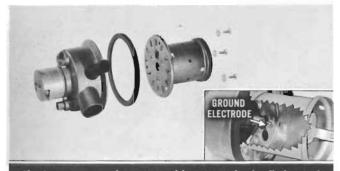
If mixer cup must be removed because of a badly burned shell, a burned-away ground electrode, or to test or service the fuel section of the burner housing, remove three screws which secure cup to housing. Separate mixer cup and gasket from housing.
