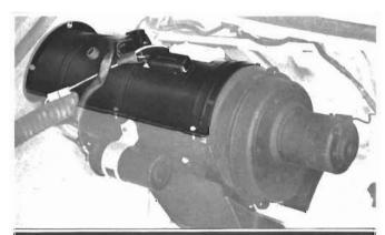
BURNER ASSEMBLY: To get to the burner assembly, the top half of the heater case must be removed as follows:
