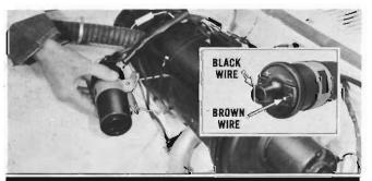
COIL: When replacing coil be sure brown wire is connected to the primary negative (—) terminal and the black wire connected to the primary positive (+) terminal. NOTE: This is a special high voltage coil. Do not attempt to replace it with a standard automotive coil.
