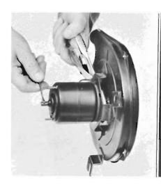
To replace cam, hold other end of motor shaft with pliers and unscrew cam counterclockwise from threaded end of shaft. Install new cam by reversing removal procedure.
