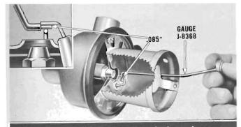
Use other end of Gauge J-8368 to check gap between electrodes. This end of gauge is .085" thick. Bend ground electrode only to adjust gap. Recheck alignment of ground electrode to fuel nozzle.
