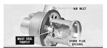
Install mixer cup and gasket, aligning spark plug openings in mixer cup and burner housing. The full circumference of the center opening in the mixer cup MUST seal firmly against the tapered end of the fuel nozzle. Check by looking through air inlet. There should be <u>no</u> light visible around nozzle.
