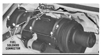
Remove two screws holding upper half of heater case to fender. Remove three strap screws. Remove two top screws holding ventilator blower housing to heater case. Separate fuel solenoid wire connector.
