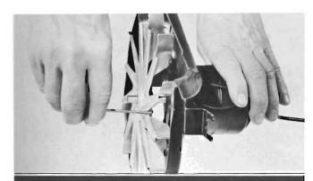
Remove ignition unit from end of motor as shown earlier. Remove outer half of blower case and loosen Allen head screw in inner side of fan hub. Pull fan off shaft.
