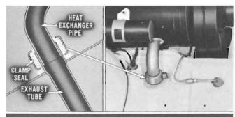
Install the heater exhaust tube, making sure it projects up into the luggage compartment. This locates the heat exchanger pipe correctly inside the exhaust tube, and the clamp and clamp gasket can now provide a good seal. Tighten the clamp securely. Install the metal shield.
