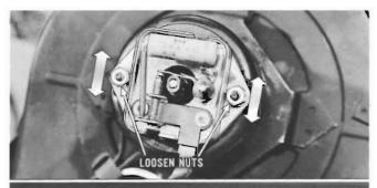
If point gap readings are within .010" of each other but either is below .012" or over .021", try to bring both gaps within desired reading by loosening the two ignition unit mounting nuts and shifting assembly slightly as permitted by bolt hole clearance.
