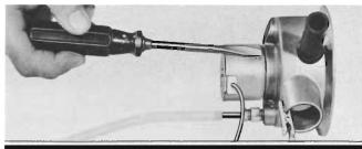
If no fuel sprays from nozzle, the solenoid coil, fuel inlet screen, fuel valve or nozzle assembly could be at fault. Check the solenoid coil by opening and closing the solenoid electrical circuit while holding the blade of a screw driver close to the solenoid cup. A good coil will attract the blade when the coil is energized. If solenoid coil is not functioning, stop engine and replace coil as follows:
