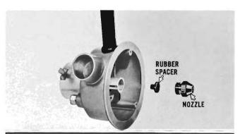
If the cause of fuel blockage is not due to an inoperative solenoid, all other components of the fuel section should be removed and inspected. Remove fuel nozzle and rubber spacer.
