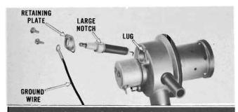
Install spark plug with gaskets and rubber sleeve in burner housing. The large notch in the spark plug porcelain indexes with a lug in the burner housing to provide correct electrode alignment. Ground wire should be installed between attaching screw and retaining plate as shown.
