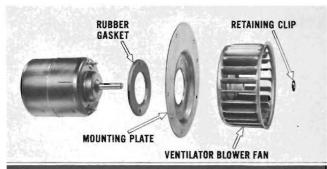
To remove fan, loosen retaining clip (or set screw) whichever is used. Install new blower motor or fan as required. Reverse procedures to assemble and install. (Use the alignment marks to assist in proper reassembly and installation.)
