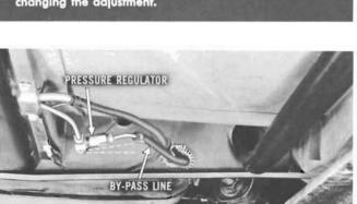
PRESSURE REGULATOR: When installing a new pressure regulator make certain the by-pass line is at or slightly above horizontal, so air bubbles or vapor will vent to the fuel tank.
