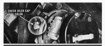
Distributor Identification: When tuning Powerglide-equipped engines, check the distributor oiler cap. A BLACK cap indicates the centrifugal advance mechanism is the intermediate or late type and has a specific advance curve. A <u>copper-plated</u> cap indicates the engine is the high-performance unit.
