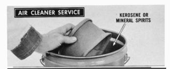
Proper maintenance service of the air filter element (every 2,000 miles) is extremely important to provide maximum engine life and a minimum of fuel consumption. Replace torn or ripped elements. Thoroughly clean the element in clean kerosene or mineral spirits. CAUTION: Never use a hot degreaser or solvents containing acetone or paint thinner.
