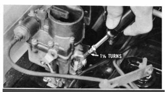
Turn the idle mixture screws on both carburetors <u>in</u> until they are lightly seated, then back off 1½ turns. This is an approximate setting. Connect the tachometer and start engine.
