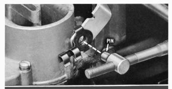
Rotate the swivel on the accelerator rod to align the swivel pin to the cross shaft lever hole. The pin should enter the attachment hole without forcing. Connect linkage and make sure clip is firmly installed.
