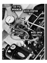
Remove the air cleaner and hoses. Block or hold the accelerator rod in the wide-open throttle position. Crank the engine over at least FOUR compression strokes. Compression should read at least 130 psi. Variation between the highest and lowest reading cylinders should not be more than 20 psi.
