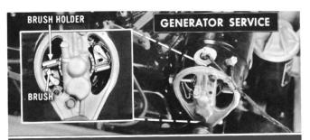
Check the brushes for free movement in the holders. Brushes which are less than half of their original length (15.6") should be replaced. Clean oily or dirty commutators using a soft, clean rag. Worn-out brushes or a scored commutator should be corrected as shown in the Corvair Shop Manual, Pages 8-11 to 8-16.
