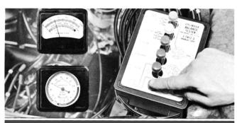
Rotate the fast idle cam to obtain a constant 1500 rpm. Depress the panel buttons in the order shown on the overlay card. Note vacuum and rpm for each pair or bank of cylinders being tested. Equal gauge readings indicate that the engine can be successfully tuned.
