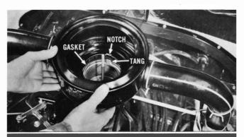
Clean the air cleaner assembly and cover. Install a new gasket on the air horn casting. Install the unit so that the notch indexes with the tang.
