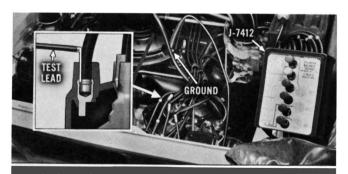
Cylinder Balance Test: This test quickly compares power output of pairs or banks of cylinders through rpm and vacuum readings. Insert the test lead prongs of J-7412 into the distributor cap spark plug sockets. Ground the unit. CAUTION: Do not pierce the wires.
