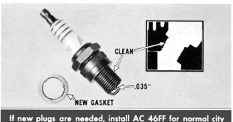
If new plugs are needed, install AC 46FF for normal city driving. For drivers who travel at high speeds or on long trips, use colder heat range spark plugs, AC 44FF. Gap new or cleaned plugs .035". ALWAYS use new gaskets and make sure the cylinder head and plug threads are clean.
