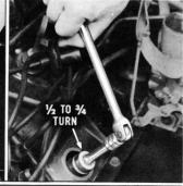
Screw the plugs all the way down until they seat on the gasket finger-tight. Tighten the plugs ½ to ¾ turn further to provide the proper seal. If a torque wrench is used, tighten plugs to 20 to 25 foot-pounds.
