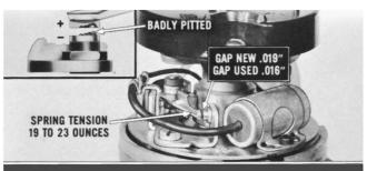
Distributor Points: Install new points if badly pitted. If mildly rough, use a clean point file. Never attempt to file smooth by removing all of the roughness. Gap new points .019" — used points .016". Dwell should always be checked (33°). See Part II for dwell tests. NOTE: Spring tension should be 19 to 23 ounces.
