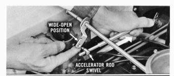
Disconnect the accelerator rod swivel from the cross shaft lever. Hold the lever in the wide-open throttle position. With the accelerator pedal held all the way down to the floor mat (a pedal depressor tool may be used) grasp the accelerator rod and push firmly toward the front of the car to remove all slack in the linkage.
