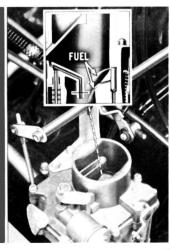
If only one stream is noted from either carburetor and the discharge openings are not plugged, install the Carburetor Accelerating pump unit, Part Number 7017524.
