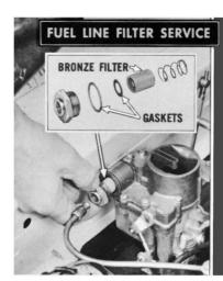
Disconnect both fuel lines and remove both large inlet nuts. Remove the sintered bronze filters, the filter gaskets and springs. Blow compressed air in the opposite direction to fuel flow to remove loose particles and reinstall parts as shown.
