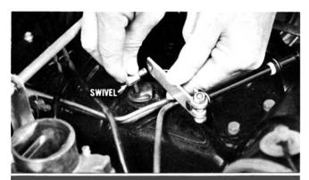
If the measurement is incorrect, disconnect the swivel and adjust the length of the rod. Reinstall swivel and recheck.
