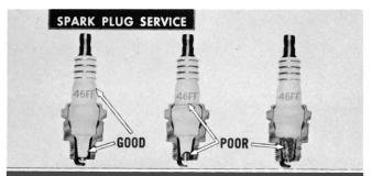
If the cylinder balance test results were good or if the compression readings were normal, carefully inspect all plugs to determine if they will fire properly until the next tune. This requires good judgment, experience, mileage information and, if possible, a knowledge of owner driving habits.
