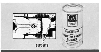
Unusually high compression may be caused by excessive combustion chamber deposits. These deposits can be inexpensively removed with GM Carburetor and Combustion Chamber Cleaner, Part Number 3727702. Follow the instructions on the can label.
