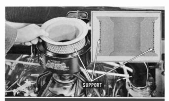
Install the filter element into the screen support. The upper and lower flanges must provide a good seal to the air cleaner and to the cover when installed.
