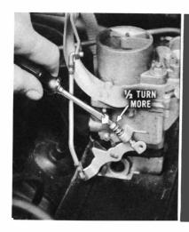
Starting with the RIGHT carburetor, turn the idle speed screw in until it just touches the throttle shaft lever, then turn clockwise an additional ½ turn. Repeat this procedure for the left carburetor.
