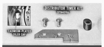
All engines teamed with Powerglide which have a <u>cadmium</u>-plated oiler cap should have the distributor modified. Distributor Timer Kit, Part Number 3784096, is available for field use and contains installation instructions. After installation of this kit the oiler cap <u>must</u> be painted black for future identification.
