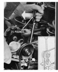
If belt needs adjustment and a tension gauge is not available, loosen the idler bracket bolt and nut. Insert a 16" (over-all length) screw driver between the pulley and bracket with the blade tip against the engine boss. Hold a 25-pound pull, then tighten the attaching nut and bolt.
