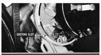
Vacuum Control Setting (all models): The vacuum control is properly set when the 23-degree mark on the calibrated scale is aligned to the edge of the casting slot on the distributor body.
