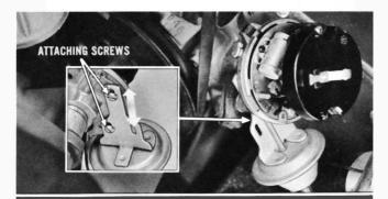
If the vacuum control setting has changed, loosen the two attaching screws on the underside of the distributor body. Slide the unit as needed to align marks. Tighten screws securely.
