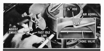
Choke Unloading: Hold or block the accelerator pedal to the floor mat (through detent on Powerglide models). Using a suitable ¼" diameter rod, adjust the swivel on the fast idle link to obtain ¼" clearance between the top of the choke valve and the upper wall of the air horn.
