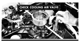
With the engine normalized, turn ignition switch OFF. Pull up on the thermostat rod (not the cooling air ring) until the bellows is stopped within its mounting bracket. The opening of the air valve directly opposite the hinge should measure 1½".
