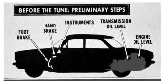
To protect the mechanic and dealership and to prevent damage to the engine, car interiors, and equipment, always check brake operation (including parking brake), instruments and telltale lights, engine and automatic transmission oil level. Install fender and seat covers.
