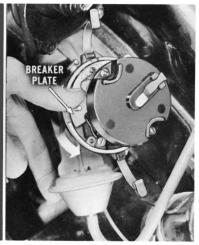
If either the rotor or breaker plate does not return promptly to its retarded position, remove the distributor from the engine and correct the cause of binding or stiffness before proceeding with the tune-up. Improper operation of either of these spark control units will directly affect distributor timing, the degree of spark advance, and cause sluggish engine performance.
