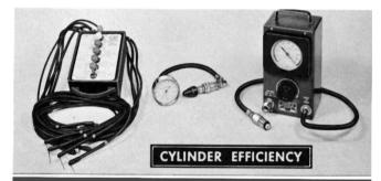
Maximum results from the tune-up depend on peak operating efficiency of individual cylinders. Three practical methods which can be used to provide this information are: the cylinder balance tester, the compression gauge, and the cylinder leakage tester.
