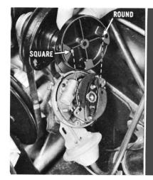
When reassembling or installing a rotor, note the round and square dowels for proper positioning.
