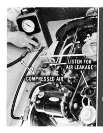
Cylinder Leakage Test: This test will help locate the exact cause of low compression through the use of compressed air. Air leakage into manifolds with the piston at TDC (compression stroke) means valve trouble. Leakage into the crankcase indicates faulty rings. Air escaping between head and piston cylinder means a defective head gasket.
