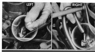
Disconnect the vacuum spark control hose from the right carburetor and the spark control plastic cap from the left carburetor. Rotate the fast idle cam to produce a constant 1200 rpm. A higher or lower rpm will reduce the accuracy of the balance settings.
