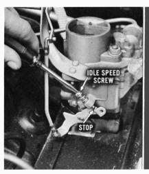
With the engine not running, make sure the choke is in the full OFF position. Back off both idle speed screws until they clear the throttle shaft lever stops.
