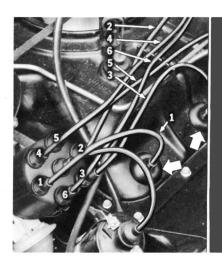
Connect all plug wires and plug covers. Improperly installed covers reduce the efficiency of the air pressure cooling system, and can cause engine overheating. Check plug wire routing. Cross firing may occur if improperly positioned.
