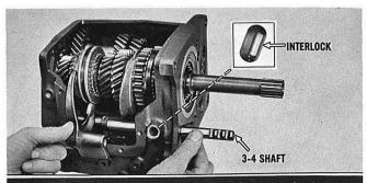
Tap the 3-4 shaft out of the case, and remove the 3-4 shift fork. Tip the case or use a magnet to remove the interlock from the detent channel. NOTE: The 3-4 shaft, 1-2 shaft and the reverse shaft can be removed from either end of the case.
