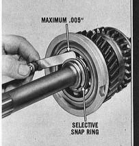
Install the selective snap ring. Measure the clearance between the rear face of the rear bearing and the snap ring. Maximum allowable end play should be .005". This snap ring is available in three thicknesses, .084" — .087" — .093", to obtain the correct clearance.
