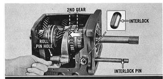
Shift the 1-2 synchronizer clutch sleeve full forward into 2nd gear. Drive the roll pin out of the 1-2 shift fork and shaft. Tap the shaft out of the case and remove the shift fork. Keep the interlock pin with the shaft. Remove the second of the two interlocks.
