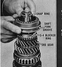
Install the 3rd-speed gear with the clutching • teeth upward. Place one of the 3-4 blocker rings on the cone surface of the 3rdspeed gear. Install the 3-4 synchronizer clutch with the shift fork groove downward. Turn the blocker ring until the notches engage the keys. Install the special snap ring.
