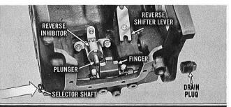
Remove the reverse shifter lever from the pivot pin and the drain plug. Remove the selector shaft finger and tap the selector shaft out of the rear of the case. Remove the reverse inhibitor with its plunger by removing the cap screws. This completes the disassembly of the case. The reverse inhibitor on . . .
