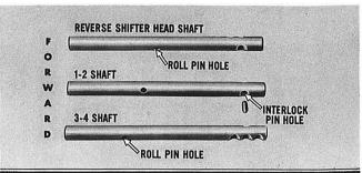
Before installing the 3 main shifter shafts, let's identify each. The reverse shifter head shaft has the roll pin hole almost centered on the shaft. The 1-2 shaft has an interlock pin hole drilled through the end of the shaft. The 3-4 shaft roll pin hole is nearest the forward end of the shaft.
