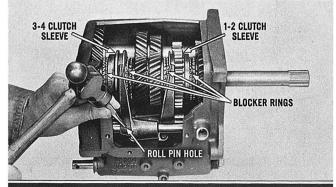
Shift the 1-2 and 3-4 synchronizer clutch sleeves into neutral position (all blocker rings will be visible). Drive the roll pin out of the 3-4 shift fork and shaft.
