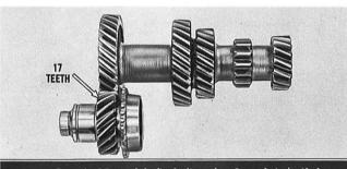
. . . Corvair 95 models (including the Greenbrier). If the clutch gear has 16 teeth, it must be replaced during assembly with part number 3785454, which has 17 teeth, in order for the countergear and clutch gear to mesh properly. All other mainshaft gears will mesh satisfactorily with the relieved countergear.
