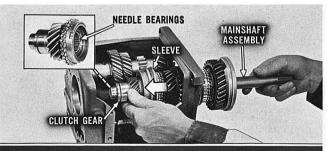
Shift the 3-4 synchronizer sleeve full forward (4th gear). Grasp the clutch gear and the rear of the mainshaft, and remove the complete mainshaft assembly from the case. NOTE: Be careful to prevent the clutch gear from separating from the mainshaft. There are 70 needle bearings inside the bore of the clutch gear.
