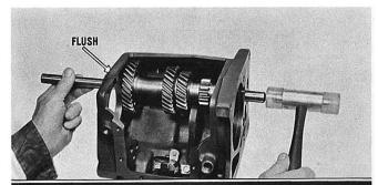
Push the countergear shaft into the rear of the case by hand. Then tap the countershaft with a soft-faced hammer until the shaft is flush with the front face of the case. The shaft is a slight press fit at the forward end. Turn the countergear by hand to check ease of rotation. Place the reverse shifter lever on the pivot pin with the tapered end inward. Position the reverse-idler gearshift fork in the case with its pin towards the front of the case, and engage the pin with
