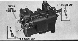
Install both the 1-2 and the 3-4 detent balls, springs, nylon washers and detent caps. The 1-2 cap has the longer thread length. Install the small snap ring in the inner diameter of the clutch gear. This snap ring is a bottoming stop for the clutch shaft.
