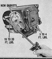
20 ft. lbs. This completes the overhaul of the four-speed transmission.
