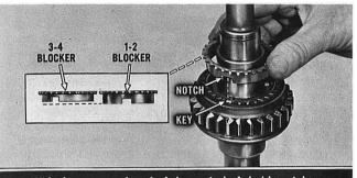
With the rearward end of the mainshaft held upright, position one of the 1-2 blocker rings in the synchronizer assembly. Engage the notches with the keys. NOTE: The 1-2 and the 3-4 blockers are slightly different. The 1-2 blockers have longer hubs.
