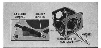
Insert one of the detent springs and a ball into the 3-4 detent channel. Slightly depress the ball and spring with a drift punch and, at the same time, insert the reverse shifter head shaft into the case past the spring-loaded ball. The two detent notches face towards the detent ball.
