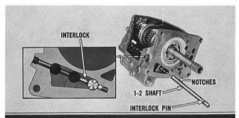
Shift the synchronizers to their neutral position, then install one of the interlocks in the 3-4 detent channel. Insert the interlock pin in the 1-2 shaft, and install the shaft partially into the case. The three detent notches at the forward end of the shaft must face towards the reverse shifter shaft.
