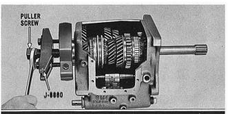
Install the clutch bearing puller plates, J-8880, into the bearing groove and the adapter plug into the clutch gear bore. Turn the puller screw slowly until the bearing is separated from the case. Remove the puller plates and adapter plug.
