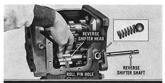
Drive the roll pin out of the reverse shifter shaft. Tap the shaft out of the case, and remove the shifter head. Remove the detent ball and spring from the bottom of the detent channel bore. NOTE: All detent springs and balls are identical.
