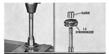
Further disassembly of the mainshaft is not required if the assembly is undamaged. However, when necessary, press the mainshaft out of the 1st-speed gear sleeve and the 1-2 synchronizer hub. This completes the disassembly of the mainshaft.
