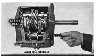
Engage the 3-4 shift fork with the synchronizer sleeve. Insert the shaft through the shift fork, and align the roll pin holes. Install the roll pin.
