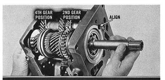
Shift the 3-4 synchronizer sleeve forward into 4th-gear position and the 1-2 synchronizer sleeve into 2nd-gear position. Then, insert the mainshaft through the case until the rear bearing retainer is flush with the rear face of the case. The clearance hole in the retainer and case must align.
