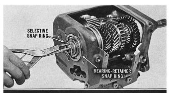
Install the front bearing (with snap ring) into the case, and tap around the outer edge of the bearing race until the snap ring seats against the case. Install the selective snap ring in the clutch gear groove.
