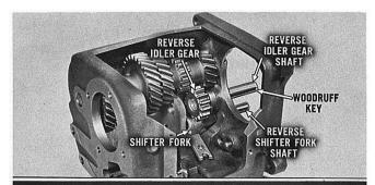
Remove both the reverse shifter fork shaft and the reverse idler gear shaft by tapping the shafts out of the case. The Woodruff key in the end of the reverse idler gear shaft prevents the shaft from rotating. Remove the reverse idler gear and the shifter fork.
