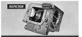
Wash the transmission case and all individual components in a good commercial cleaning solvent or clean kerosene. Air-dry, using compressed air. Inspect the case for cracks, especially near the front- and rear-bearing bores. Clean all old gasket material from surfaces of case and covers.
