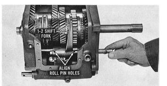
Engage the 1-2 shift fork with the 1-2 synchronizer sleeve. This shift fork is easily identified by the through gate. Push the shaft through the fork and align the roll pin holes. Install the roll pin.
