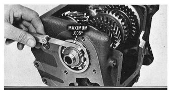
Measure the clearance between the bearing and selective snap ring. Maximum allowable clearance should be .005". This snap ring is available in three thicknesses, .084" — .087" and .093", to obtain correct clearance.
