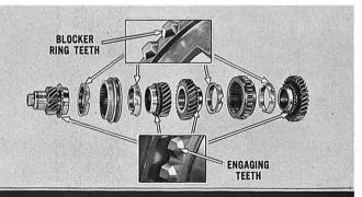
Inspect all blocker ring teeth and the engaging teeth of the synchronizer sleeves and matching gears. The teeth must be sharply defined and not rounded. Install new parts as necessary. Turn the front and rear bearings by hand to check for a binding condition or rough spots. To replace the rear bearing, support the retainer on press plates, then expand the snap ring as the bearing is pressed out of the retainer. Reverse the procedure for installation.
