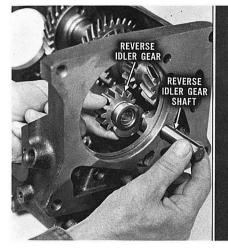
With the reverseidler gearshift fork fully forward, install the reverse idler gear to the shift fork as shown. Insert the reverse idler gear shaft partially into the case.
