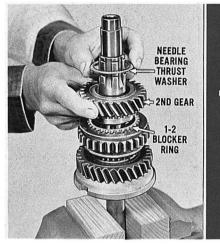
Clamp the mainshaft in the vise so that the forward end is up. Install the second of the 1-2 blocker rings, and engage the notches with the keys. Install the 2nd-speed gear with the clutching teeth downward. Place the needle-bearing thrust washer on the 2nd-speed gear.
