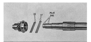
Remove the 37 outer needle bearings and the 33 inner needle bearings from the clutch gear bore. All are  $\frac{3}{22}''$ in diameter and  $\frac{1}{2}''$  long. Inspect the bearings, the clutch gear and the pilot end of the mainshaft for galling or excessive wear. Install new parts as necessary.
