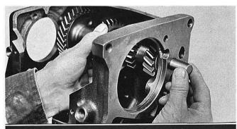
Insert the countergear assembly through the rearbearing opening, and carefully lift the assembly into position between the thrust washers. Then, remove the two short pieces of rod.
