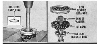
Remove the rear-bearing selective snap ring. Support the 1st-speed gear on suitable blocks, then slowly press the mainshaft out of the bearing bore. To avoid damage, the blocker ring must remain clear of the supports. Remove the 1st-speed gear thrust washer, the 1st-speed gear and the 1st-gear blocker ring.
