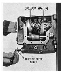
Temporarily attach the front bearing retainer to the case with two cap screws. Test the operation of the shift forks, synchronizers, and the general shifting ability of the
