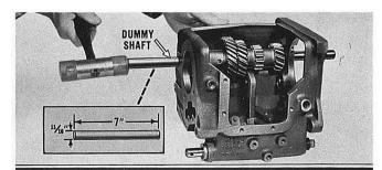
Using a drift punch, tap the countergear shaft a short distance out of the rear of the case. Then, using a locally made dummy shaft, tap the countergear shaft all the way out. The dummy shaft will keep the 92 needle bearings inside the countergear bore from falling out of position as the countergear shaft is removed.
