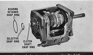
Remove the bearing retainer snap ring, the clutch bearing selective snap ring and the clutch shaft bottoming snap ring.
