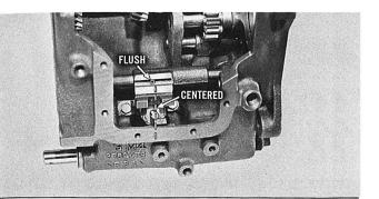
Install the roll pin until it is flush with the bottom face of the sliding gate. Move the shaft forward until it drops into the detent which centers the shifter gate opening with the inhibitor plunger. This will permit installation of the 1-2 shaft.
