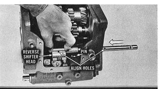
Engage the pin of the reverse shifter head with the yoke of the reverse shifter lever. Then, push the shaft into the case and through the bore of the shifter head until the roll pin holes align.
