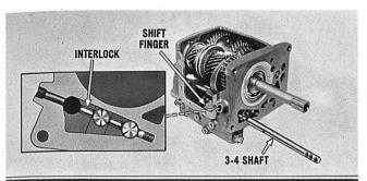
Drop the remaining interlock into the detent channel, and insert the 3-4 shift fork shaft partially into the case. The three detent notches should be up, facing away from the 1-2 shaft. If necessary, move the selector shaft so that the shift finger drops into the opening in the 1-2 shift fork gate.
