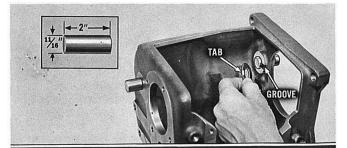
Coat both countergear thrust washers with petroleum jelly, and position each against the case with the tabs engaged in the case grooves. Two short pieces of rod (<sup>11</sup>/<sub>16</sub>" O.D. x 2" long) inserted into the shaft bore, as shown, will help to hold the washers in position during countergear installation.
