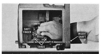
Coat the selector shaft and seal lips with petroleum jelly, and insert the shaft through the rear of the case. Attach the shift finger with cap screws. Bend the lock tangs against the heads of the cap screws. Install the drain plug.
