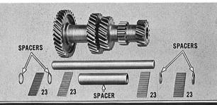
Remove the 92 needle bearings from the countergear (four sets of 23 each). All are  $\frac{7}{64}$ " in diameter and  $\frac{3}{4}$ " long. Inspect the bearings, spacers and the countergear shaft and bore for galling or excessive wear. Install new parts as necessary. Use petroleum jelly and the dummy shaft to assist in their installation.
