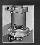
Caution should be observed to prevent damage to the bearing and retainer during removal and installation. A  $2\frac{3}{4}$ " O.D. sleeve will assist in removing the bearing and prevent damage to the new bearing during installation. This completes the inspection procedures.
