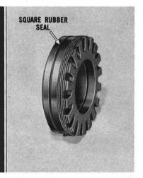
Install new square rubber seal on side adjusting sleeves. Coat threads with a non-hardening pipe compound, then install loosely in position to align differential side bearings.
