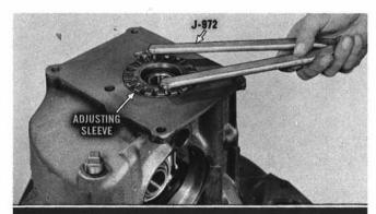
Remove Differential Carrier top cover and gasket. Then, remove lock tab screw and lock tab, holding pinion adjusting sleeve. Use Tool J-972 and unscrew adjusting sleeve.
