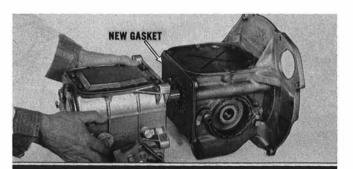
To join 3-speed transmission and carrier, apply petroleum jelly to new gasket and mount on either transmission or carrier. Carefully engage splines of transmission mainshaft with pinion shaft splines and draw units together. Install attaching bolts and torque 24 to 32 foot-pounds.
