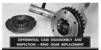
Use a suitable tool and make alignment marks in differential case and cover. Remove the six bolts holding case together. Use soft hammer and tap ring gear from case. For ring gear replacement only, further disassembly is not required.
