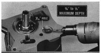
With shaft fully seated, drill a  $\frac{3}{16}$  hole at a fairly flat angle in the shaft bore just above the step in the end of the shaft. Drill  $\frac{3}{8}$  to  $\frac{1}{2}$  maximum depth to prevent breaking through into transmission.
