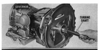
Install governor and install all four attaching bolts. Torque 24 to 32 foot-pounds. Install turbine shaft, making sure all splines are engaged. To install converter and reassemble power train, refer to Corvair Shop Manual, Page 6-11, or the film Servicing the Corvair Powerglide—Part IV, Overhaul.
