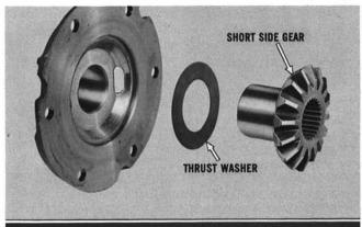
Continue by removing short side gear and thrust washer from differential case.
