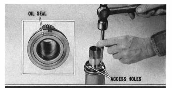
Powerglide-equipped units use a pinion rear oil seal in the stator shaft bore. If damaged, drive out old oil seal with pin punch through access holes as shown.
