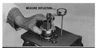
Without disturbing setting of indicator, carefully lower support on governor gear as shown. Measure the needle deflection from ZERO, then refer to the following table from Page 6-10 of the Corvair Shop Manual for the required number of spacers.
