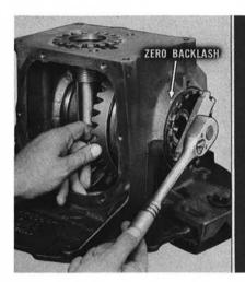
Tighten side adjusting sleeves and pinion adjusting sleeve to take up all lash. Tighten right-side adjusting sleeve until there is ZERO backlash. This is a matter of "feel." Mark carrier case and corresponding notch with a crayon.
