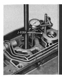
Place transmission front end down on bench and remove turbine shaft. Install a dial indicator on Support J-8364 and install 3" extension. Place support on rear pump cavity surface as shown, with indicator tip resting on planet carrier hub.
