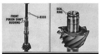
On Powerglide-equipped units, carefully chisel out front pinion shaft bushing if worn. Use Bushing Installer J-8333 to install new bushing as shown. Inspect pinion shaft seal ring on rear of pinion shaft and replace if broken.
