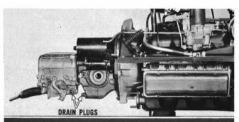
With power train mounted on transmission jack, completely drain Transaxle and clean exterior surface. To remove Powerglide Transaxles, follow steps in the Corvair Shop Manual, Page 6-7, or in the film Servicing the Corvair Powerglide — Parts III and IV, Overhaul.
