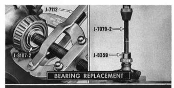
If damaged, bearings and races should be replaced as a set. To remove differential side bearings, use Bearing Puller J-7112 with Pilot J-8107-2 as shown. Clamp differential case in vise and pull bearings. Replace bearings using J-8359 and Handle J-7079-2 as shown.
