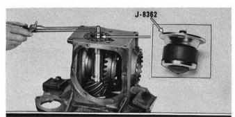
Tighten pinion bearing adjusting sleeve to just remove pinion bearing end play. Back off adjusting sleeve ¼ turn. Use Adapter J-8362 and measure the turning torque at the drive pinion. This represents the pre-load on differential side bearings.
