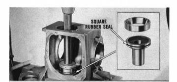
Use new square rubber seal on outer bearing shaft. Place carrier in press as shown. Make sure inner bore of carrier is thoroughly cleaned. Install new bearing shaft and bearing race using Installer J-7137 so cup is flush with inside of carrier case.
