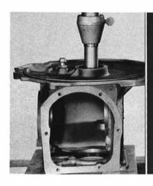
If rear pinion race is damaged, remove by placing carrier in press and pressing directly on clutch release bearing shaft or stator support as shown. Shaft or stator support and bearing race will come out together.
