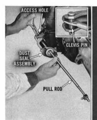
To remove Manual Transmission units, lower unit so differential carrier just rests on a flat surface. Remove two screws holding clutch pull rod dust seal assembly to clutch housing. Remove dust seal assembly. Remove the clevis pin retainer: then through access hole in clutch housing, pull out clevis pin holding clutch pull rod to clutch fork, and remove pull rod.
