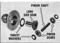
Use a small diameter punch and drive out pinion shaft retainer pin. Then remove pinion shaft, pinion gears and thrust washers. Remove long side gear and thrust washer.
