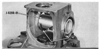
Continue by placing Gauge Cylinder Adapters J-6266-18 in each side bearing adjusting sleeve bore so they rest on machined portion of bore. Place Gauge Cylinder J-6266-01 on adapters with plunger and mounting post in a horizontal position.
