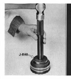
Install new race using Driver J-8148. Seal the drilled holes with lead balls similar to small fishing line sinkers. To remove pinion shaft front and rear bearings, use Puller Plate J-8331 and mount in Holder J-358-1 as shown.
