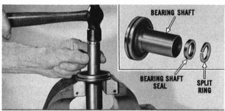
On Manual Transmission models, check clutch release bearing shaft seal for damage. To replace, remove split ring and drive out old seal as shown. Use a suitable tool and install new seal, open face inward, and tap until bottomed. Reinstall split ring.
