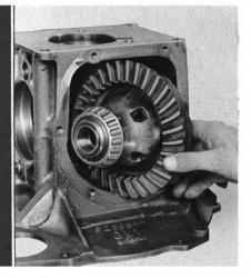
With the main components out of the carrier, clean and carefully inspect for wear. Pinion bearings will normally have a uniform frosted appearance. Unusual wear at either end of rollers indicates improper pre-loading, either too loose or too tight. Make sure races aren't cracked or gouged. Check carrier for cracks or cross threads.
