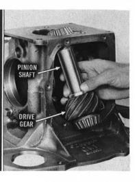
Differential case can now be removed by shifting to one side and turning at right angle so ring gear can pass through top cover opening.
