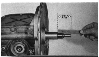
Install clutch shaft in the Transaxle. If fully engaged, the distance from end of clutch release bearing shaft to end of clutch shaft will be 2%, plus or minus 1/32".
