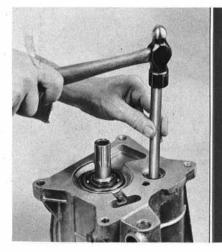
Tap countershaft with soft drift to firmly position against stakes at front of case bore. If press fit of countershaft has been lost, replace transmission case since shaft would not form an oil seal.
