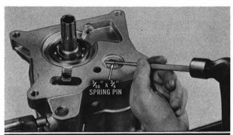
Install a ¾6" x ¾" spring pin (Part Number 454512) in newly drilled hole. Make sure pin does not protrude beyond face of transmission case.
