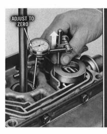
Adjust gauge to ZERO. Slowly lift gauge and note range of deflection from ZERO. If deflection exceeds .050", relocate indicator on Support J-8364 and repeat check so that deflection is less than .050".
