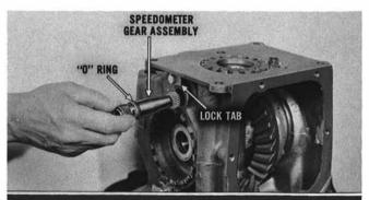
Replace rubber "O" ring seal on speedometer gear assembly and then install in carrier. Tighten lock tab. Use a new gasket under top cover and replace cover. Install attaching screws and torque 11 to 19 foot-pounds.
