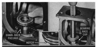
Make sure oil drain-back passage and stator shaft cavity are thoroughly cleaned. Place bearing race cup on stator shaft and press stator shaft and bearing race into carrier housing. Make sure notch on stator shaft is aligned with drain-back passage in carrier.
