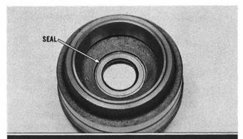
Side bearing adjusting sleeve oil seals are easily replaced by driving out with a punch. Install new seals with lip facing inward and tap into position with a soft hammer.
