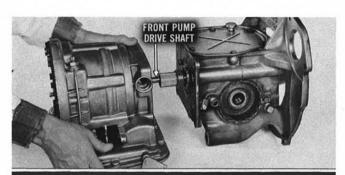
Use petroleum jelly to hold new gasket in position on either transmission or carrier. Align units on a flat surface and carefully guide front pump drive shaft through carrier to avoid damaging pinion bushings. Engage pinion shaft splines with planet carrier.
