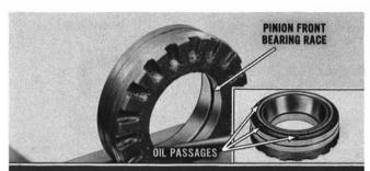
If damaged, remove pinion front bearing race by driving out with a punch. Late production models use a new-style front pinion adjusting sleeve with six drilled oil passages to lubricate pinion bearing. Replace old-style adjusting sleeves with new-style Part 3781001. Use Driver J-7137 to press new bearing race into position in sleeve.
