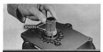
Install spacers on governor gear. Check for proper thickness by measuring with dial indicator as already shown. If spacers are correct, indicator reading will be between .011" and .038". Add or remove spacers as required to correct reading.
