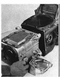
Separate transmission and Differential Carrier by removing four attaching bolts and carefully pulling two units apart. This procedure applies to both Manual and Powerglide Transaxles.
