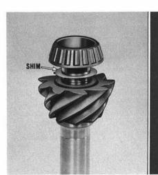
Shims are used between rear pinion bearing and pinion gear. These are for proper depth setting of pinion gear and can be re-used if pinion and ring gear are not being replaced.
