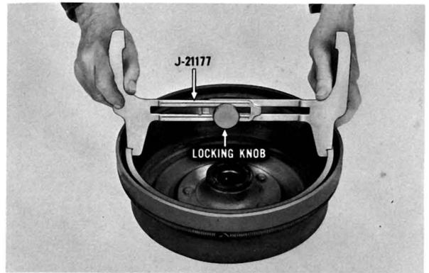
Using the special Drum-to-Brake-Shoe Clearance Gauge, J-21177, measure the brake drum diameter across the drum center line. Tighten the locking knob to hold this measurement.
