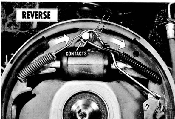
During a reverse stop, the shoes rotate with the drum until the web of the primary shoe contacts the anchor pin.
