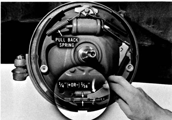
Install the primary shoe pull-back spring. Proper assembly is indicated when the bottom edge of the lever is  $\frac{1}{4}$  inch, plus or minus  $\frac{1}{16}$  inch above the center line of the adjusting screw. Check the actuating lever assembly by hand operation.
