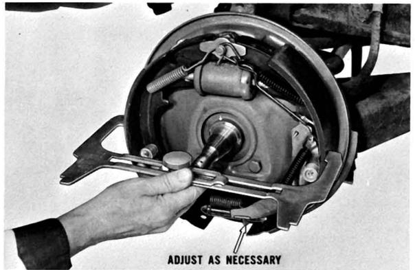
Transfer the gauge to the brake assembly with the opposite side of the gauge fitted over the shoes. Hold the actuating lever away from the star wheel, and turn the star wheel as necessary until the linings just touch the gauge.
