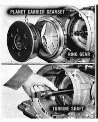
To avoid damaging converter and pinion shaft bushings when removing turbine shaft, remove planet carrier gearset and ring gear first. Then carefully pull turbine shaft from transmission.
