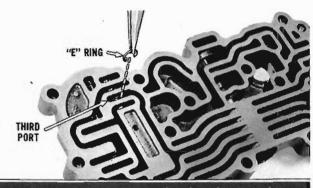
Begin reassembly by placing throttle valve in its bore and locking in place with "E" ring retainer in third port as shown. NOTE: Throttle valve must be FULLY seated in its bore to prevent being locked out of position.
