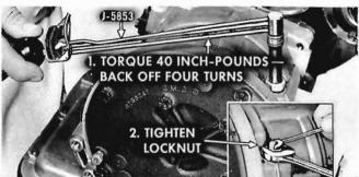
ADJUST LOW BAND: 1. Tighten adjusting screw 40 inchpounds, making certain locknut does not interfere with torque reading. Then back off adjusting screw exactly four turns. 2. Hold adjusting nut stationary while tightening locknut.
