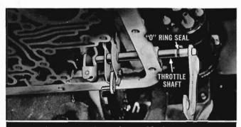
If visual inspection of case shows oil leaking past the "O" ring seal on the throttle shaft, replace seal as shown in Part II, Trouble Shooting and On-the-Car Adjustment. We are now ready to replace the valve body on the transmission case.
