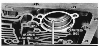
Position piston ring in bore as shown. Make sure ring is parallel with top edge of chamfer to match angle of the bore. Measure ring gap. Maximum allowable clearance is .012". If gap exceeds this measurement, use new ring. Install ring on piston and replace piston and return spring in case.
