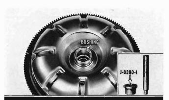
Inspect converter hub bushing. If badly scored, carefully collapse old bushing with an awl. Use the special tools shown to press new bushing into position.
