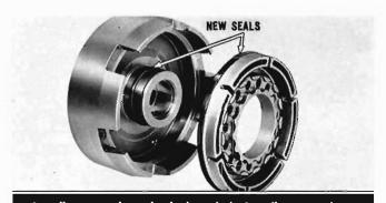
Install new seal on clutch drum hub. Install new seal on piston with lip facing toward clutch drum. Lubricate with automatic transmission fluid. Install clutch piston in drum with twisting motion being careful not to cut or roll seals out of their grooves.
