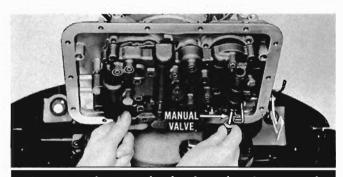
To prevent the manual valve from dropping out and possible damage, loosen the two remaining bolts slowly and evenly until manual valve is disengaged from the linkage. Pull out manual valve. Take out the two bolts and remove valve body.
