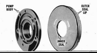
Liberally coat new inner and outer seals with automatic transmission fluid and install on reverse piston. Make sure lip of outer seal faces toward pump body. Remove rubber band from pump hub groove and install piston on pump body.
