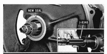
Check converter hub seal for leaks. If necessary to replace, pry out old seal with a punch. Coat outer edge of new seal with a non-hardening type sealer. Use Tool J-8340 to drive seal into position. Converter can now be installed on converter hub.
