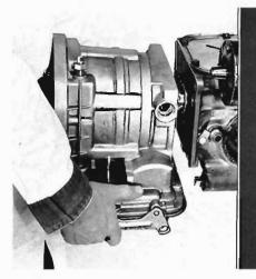
Support the transmission and take out the three remaining mounting bolts. Carefully remove transmission from the differential carrier to avoid damaging pinion shaft splines and rear oil pump bushing.
