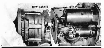
Make sure rear of transmission case is thoroughly cleaned. Use petroleum jelly to hold new gasket in position on front face of differential carrier. Carefully hold transmission in position until mounting bolts are well started. Torque bolts to 24 to 32 footpounds.
