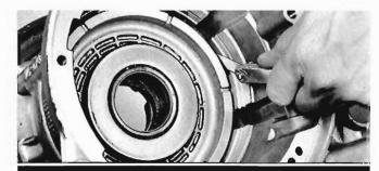
Start assembly in case using a .010-.015 feeler gauge around lip of outer seal to start seal into bore. Make sure assembly is fully bottomed. Remove guide pins and install attaching bolts. Torque 9 to 11 foot-pounds. Temporarily engage drive lugs of planet gearset in pump drive gear and rotate to make sure gears are free.
